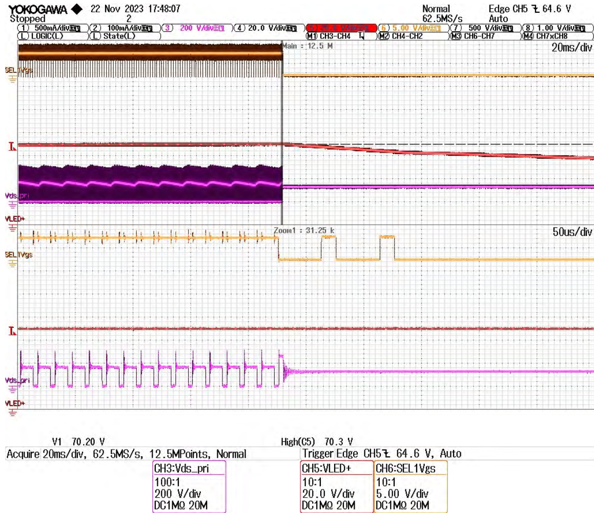
Figure 50 – LED Output OVP at Line Voltage 90 V.
