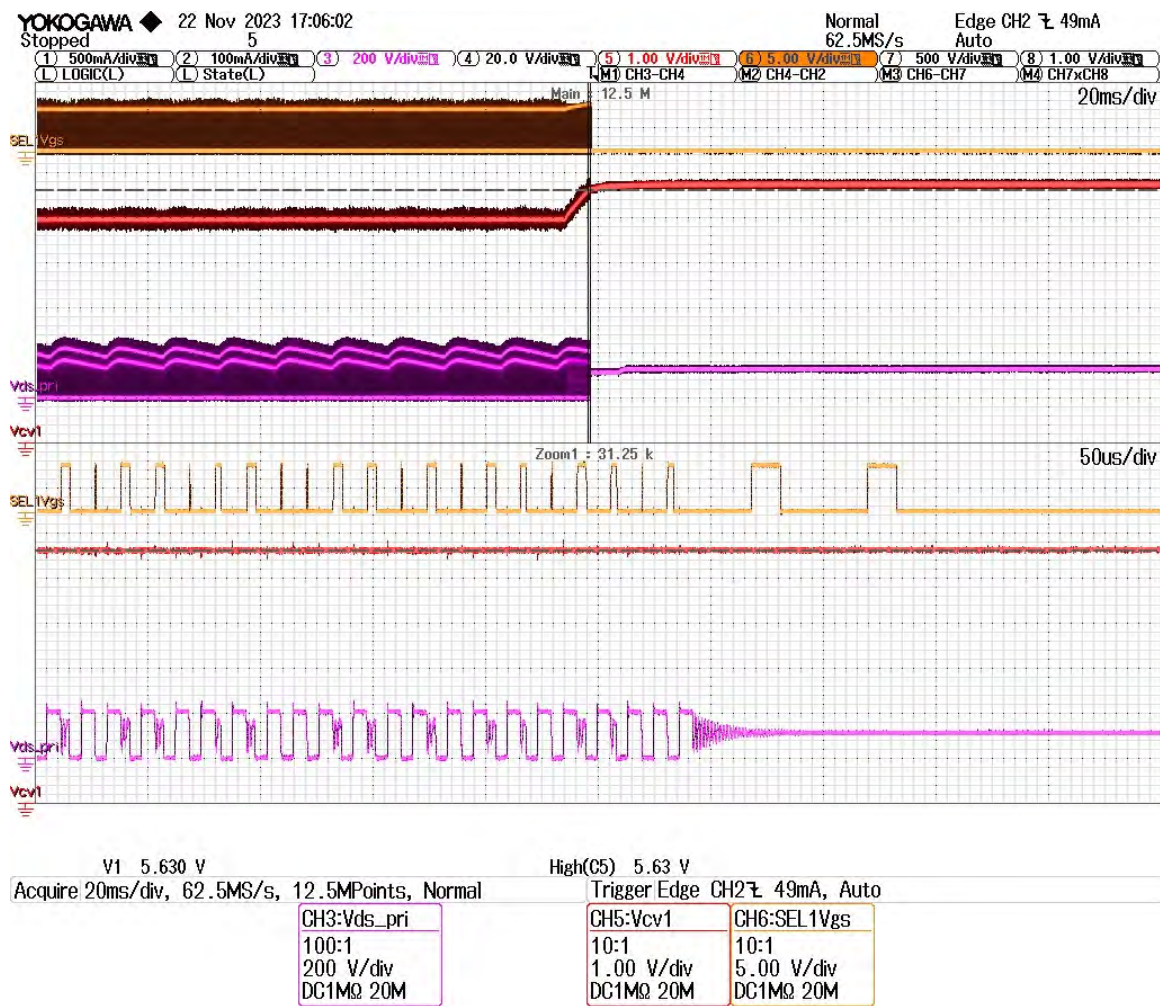
Figure 49 – CV1 Output OVP at Line Voltage 90 V.
