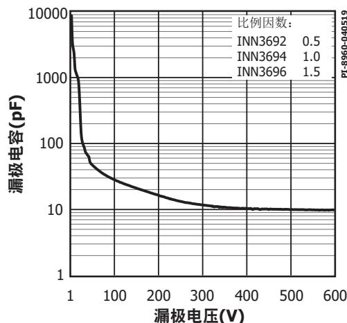
图34.  $C_{oss}$ 相对于漏极电压的变化
