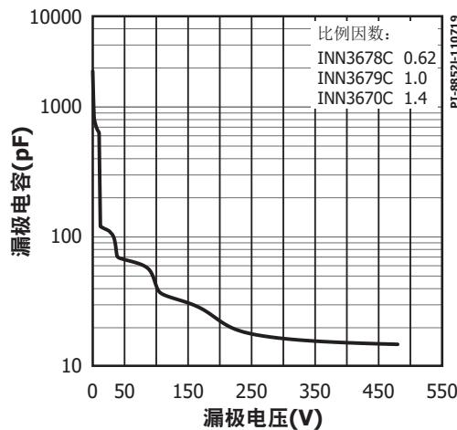
图38.  $C_{oss}$  相对于漏极电压的变化
