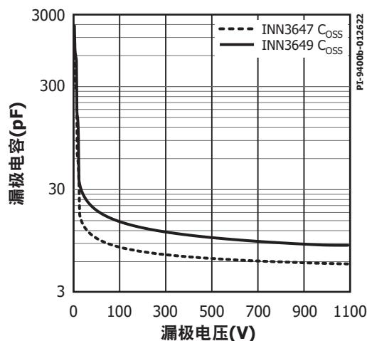
图46.  $C_{oss}$ 相对于漏极电压的变化
