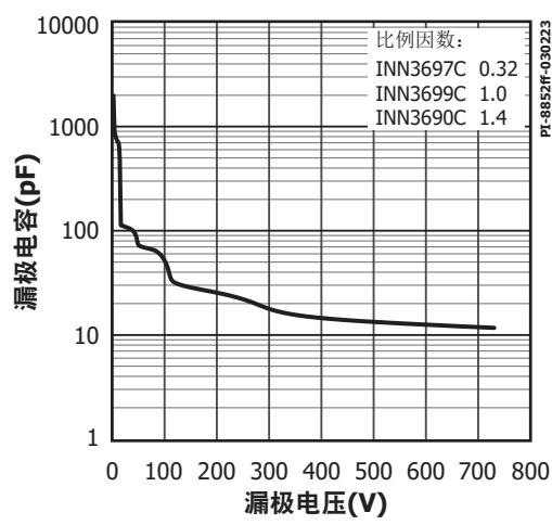
图42.  $C_{oss}$ 相对于漏极电压的变化
