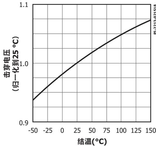
图36. 击穿电压相对于温度的变化 (不包括INN3678C/INN3679C/INN3670C/INN3647C/INN3649C)
