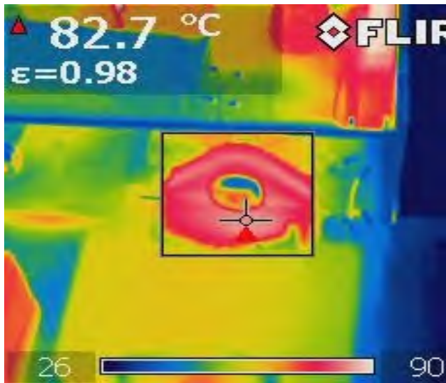
Figure 55 – LLC IC (U3), 90 VAC Input, 100% Load, Room Temperature.
