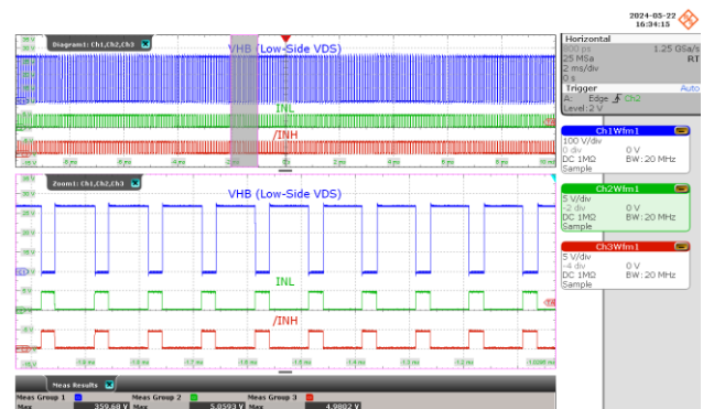
Figure 34 – INL and /INH Signals at 750 mA Load. CH1: V_{HB} , 100 V/div. CH2: V_{INL} , 5 V/div. CH3: V_{INH} , 5 V/div. Time Scale: 2 ms/div. Time Scale (Zoomed Area): 100 \mu s/div.
