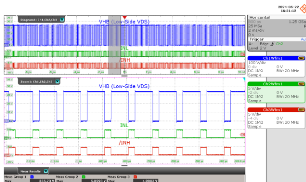
Figure 33 – INL and /INH Signals at 500 mA Load. CH1: V_{HB} , 100 V/div. CH2: V_{INL} , 5 V/div. CH3: V_{INH} , 5 V/div. Time Scale: 2 ms/div. Time Scale (Zoomed Area): 100 \mu s/div.
