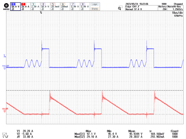
Figure 64 – SR FET Drain Voltage and Current. 900 VDC, 6.37 A Load, 25 °C Ambient. CH1: V_{DS,SRFET} , 50 V / div. CH2: I_{D,SRFET} , 20 A / div. Time: 10 \mu s / div.
