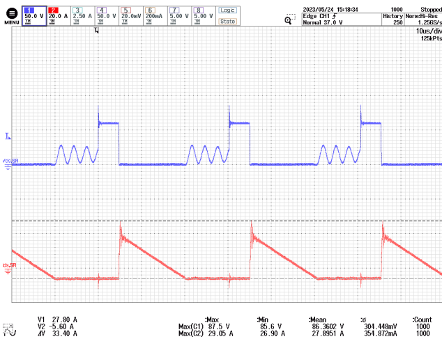
Figure 63 – SR FET Drain Voltage and Current. 800 VDC, 6.37 A Load, 25 °C Ambient. CH1: V_{DS,SRFET} , 50 V / div. CH2: I_{D,SRFET} , 20 A / div. Time: 10 \mu s / div.
