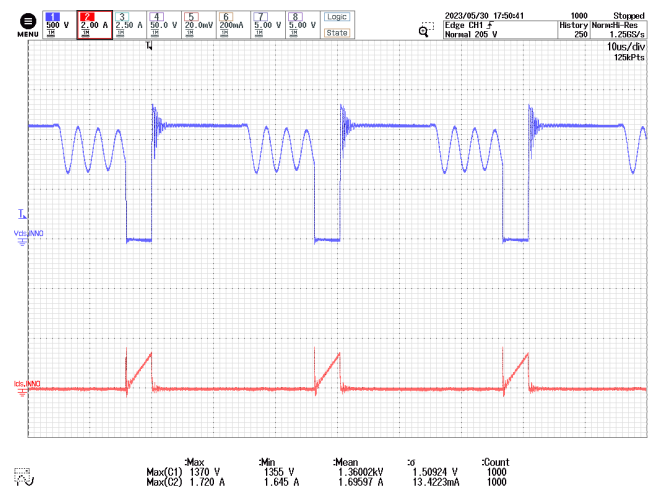
Figure 60 – InnoSwitch3-AQ Drain Voltage and Current. 900 VDC, 6.37 A Load, 25 °C Ambient. CH1: V_{DS,INNO} , 500 V / div. CH2: I_{D,INNO} , 2 A / div. Time: 10 \mu s / div.
