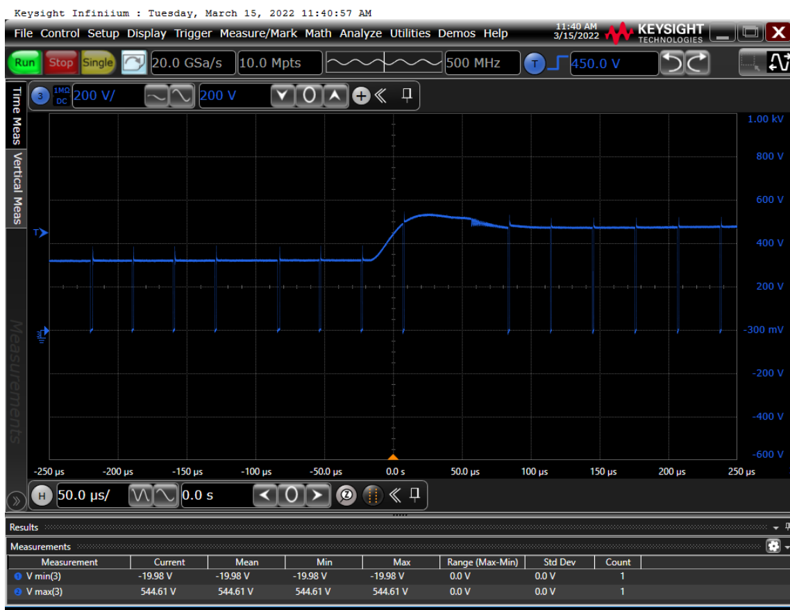
图97 - 漏极电压, 230VAC, 满载
