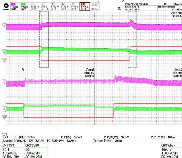
(a) 300 VDC, ICVHV = 0 A -> 2 A (100%) -> 0 A. ICV1 = 0 A. Overshoot: 520 mV (2.2%). Undershoot: -400 mV (-1.7%).
