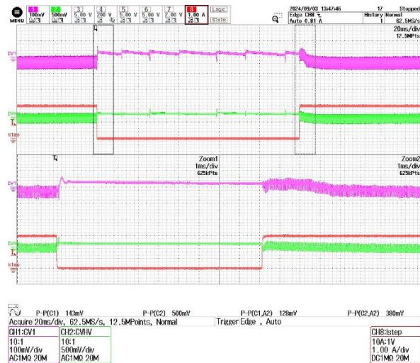
(b) 1000 VDC, ICVHV = 0 A -> 2 A (100%) -> 0 A. ICV1 = 0 A. Overshoot: 500 mV (2.1%). Undershoot: -380 mV (-1.6%).
