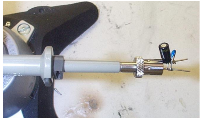
Oscilloscope Probe with Probe Master (www.probemaster.com) 4987A BNC Adapter. (Modified with wires for ripple measurement, and two parallel decoupling capacitors added)
