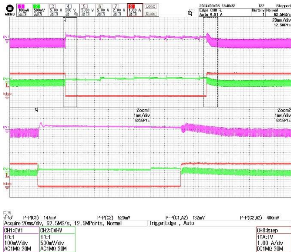
(a) 300 VDC, ICVHV = 0 A -> 2 A (100%) -> 0 A. ICV1 = 0 A. Overshoot: 520 mV (2.2%). Undershoot: -400 mV (-1.7%).
