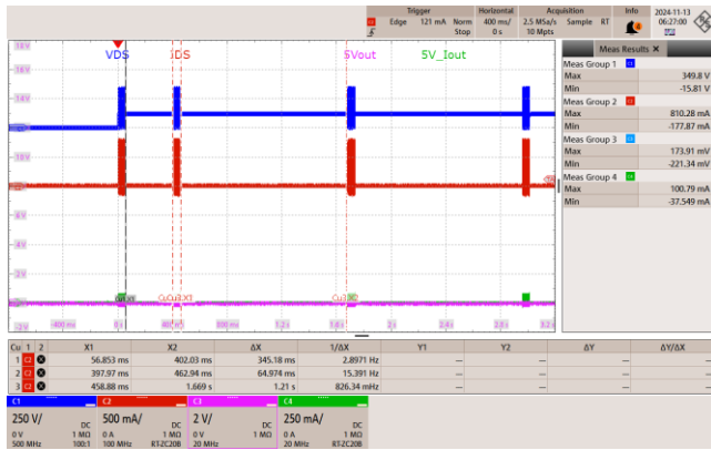
Figure 131 – 85 VAC 60 Hz 5 V Start-Up Output Short. CH1: Drain Voltage, 250 V / div., 400 ms / div. CH2: Drain Current, 500 mA / div., 400 ms / div. CH3: 5 V_V OUT , 2 V / div., 400 ms / div. CH4: 5 V_I OUT , 250 mA / div., 400 ms / div. Drain Voltage (MAX) = 350 V Drain Current (MAX) = 810 mA t_{AR(OFF)1} = 345 ms t_{AR(OFF)2} = 1.21 s t_{AR(ON)} = 65 ms
