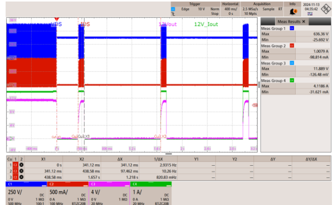
Figure 138 – 265 VAC 60 Hz. 12 V / 3.5 A, 5 V / 0.875 A. CH1: Drain Voltage, 250 V / div., 400 ms / div. CH2: Drain Current, 500 mA / div., 400 ms / div. CH3: 12 V_V OUT , 4 V / div., 400 ms / div. CH4: 12 V_I OUT , 1 A / div., 400 ms / div. Drain Voltage (MAX) = 636 V Drain Current (MAX) = 1.01 A t_{AR(OFF)1} = 341 ms t_{AR(OFF)2} = 1.22 s t_{AR(ON)} = 97.5 ms
