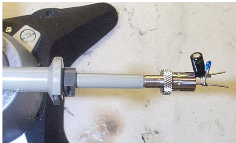
Figure 102 – Oscilloscope Probe with Probe Master ( www.probemaster.com ) 4987A BNC Adapter. (Modified with wires for ripple measurement, and two parallel decoupling capacitors added)
