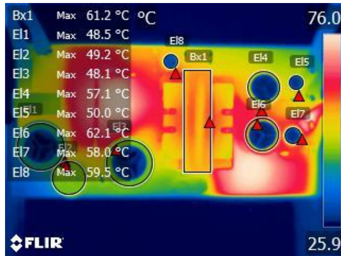
Figure 125 – 85 VAC 60 Hz Top Side Discrete Component Thermals.
