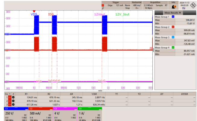
Figure 130 – 265 VAC 50 Hz 12 V Start-Up Output Short.
