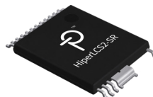
Figure 3. HiperLCS2-SR. Safety Isolation Package, InSOP-24D Top View.
