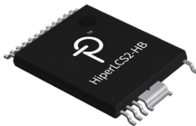
Figure 2. Primary-Side Packages. (Left) POWeDIP-20B (Right) InSOP-24C Top View.
