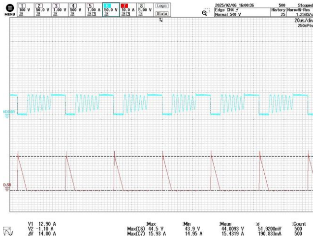
Figure 86 – SR FET Drain Voltage and Current. 200 VDC, 1.46 A Load, 25 °C Ambient. CH6: V_{DS,SRFET} , 50 V / div. CH7: I_{D,SRFET} , 10 A / div. Time: 20 \mu s / div.
