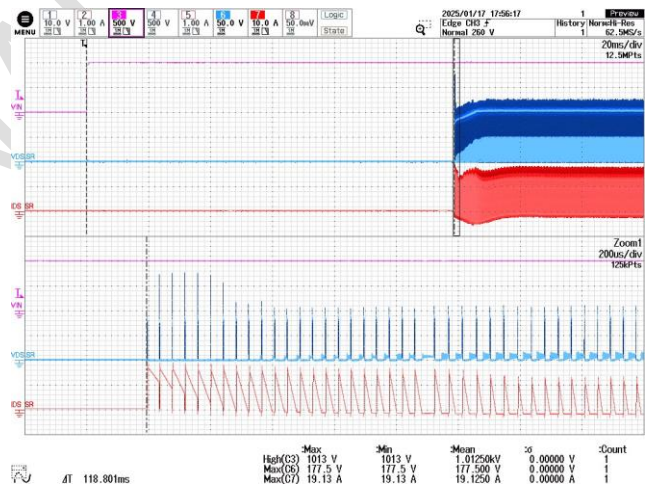
Figure 57 – SR FET Drain Voltage and Current. 1000 VDC, 16.3 Ω Load. CH3: V IN , 500 V / div. CH6: V DS,SRFET , 50 V / div. CH7: I D,SRFET , 10 A / div. Time: 200 ms / div.
