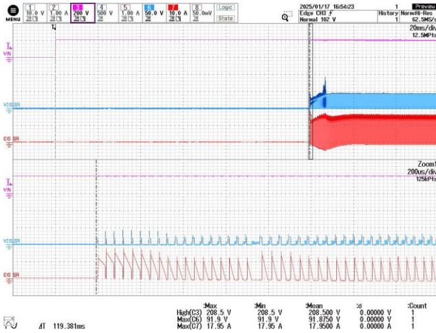
Figure 54 – SR FET Drain Voltage and Current. 200 VDC, 16.3 Ω Load. CH3: V IN , 200 V / div. CH6: V DS,SRFET , 50 V / div. CH7: I D,SRFET , 10 A / div. Time: 200 ms / div.
