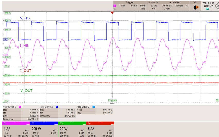
Figure 47 – LLC Stage Primary Voltage and Current, 60 V 12 A. Time Division: 10 μs/div. CH1: HB Current, 4 A/div. CH2: HB Voltage, 200 V/div. CH3: Output Voltage, 20 V/div. CH4: Output Current, 6 A/div.
