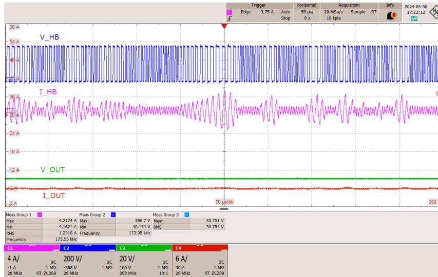
Figure 52 – LLC Stage Primary Voltage and Current, 30 V 4 A. Time Division: 10 \mu s/div. CH1: HB Current, 4 A/div. CH2: HB Voltage, 200 V/div. CH3: Output Voltage, 20 V/div. CH4: Output Current, 6 A/div.
