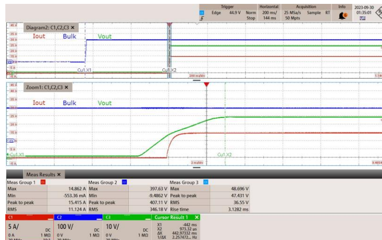
Figure 28 – Output Voltage at Start Up. 390 VDC, Full Load.
