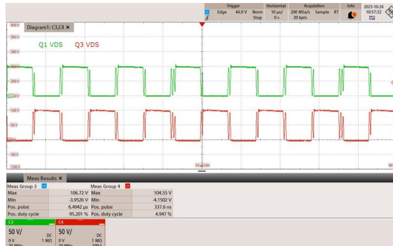
Figure 21 – Output Rectifier Peak Reverse Voltage. 400 VDC, Full Load.
