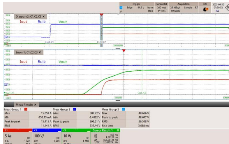
Figure 26 – Output Voltage at Start Up. 380 VDC, Full Load.
