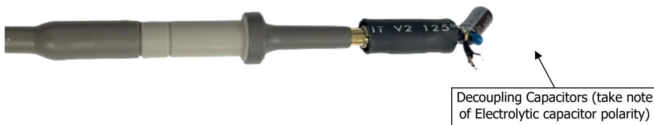
Figure 37 – Oscilloscope Probe with Probe Master 4987BA BNC Adapter (Modified with Wires for Probe Ground for Ripple measurement and Two Parallel Decoupling Capacitors Added).
