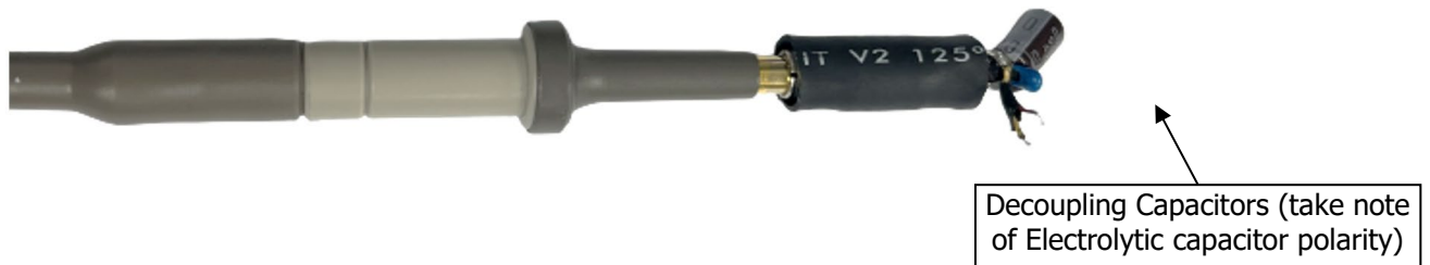
Figure 37 – Oscilloscope Probe with Probe Master 4987BA BNC Adapter (Modified with Wires for Probe Ground for Ripple measurement and Two Parallel Decoupling Capacitors Added).
