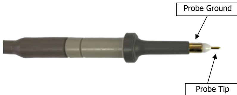
Figure 36 – Oscilloscope Probe Prepared for Ripple Measurement (Probe cover and Ground Lead Removed).
