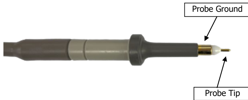
Figure 35 – Oscilloscope Probe Prepared for Ripple Measurement (Probe cover and Ground Lead Removed).
