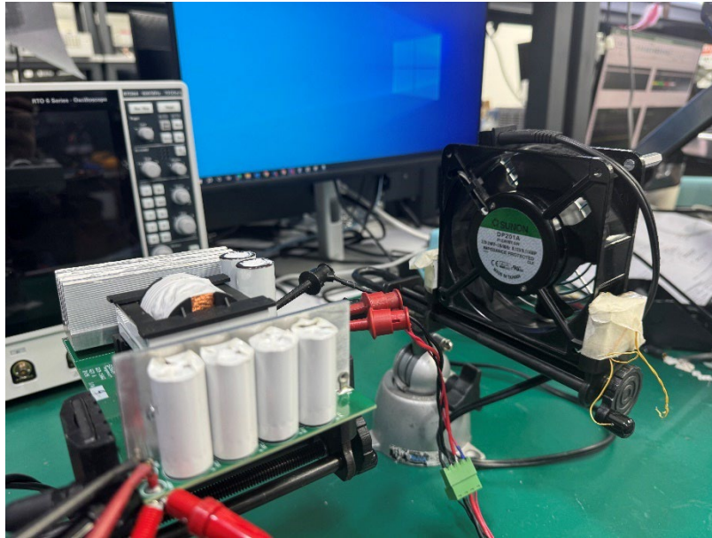
Figure 41 – Thermal Set-up with External Fan
