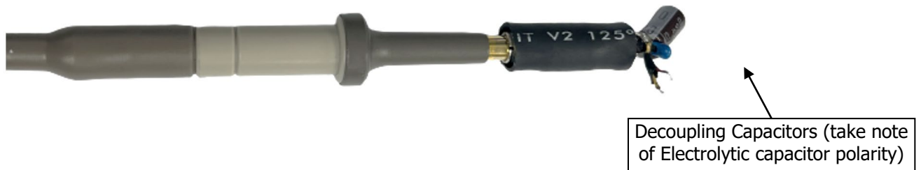
Figure 36 – Oscilloscope Probe with Probe Master 4987BA BNC Adapter (Modified with Wires for Probe Ground for Ripple measurement and Two Parallel Decoupling Capacitors Added).
