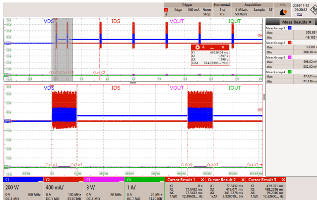
Figure 91 – 85 VAC 60 Hz. Output Short.
