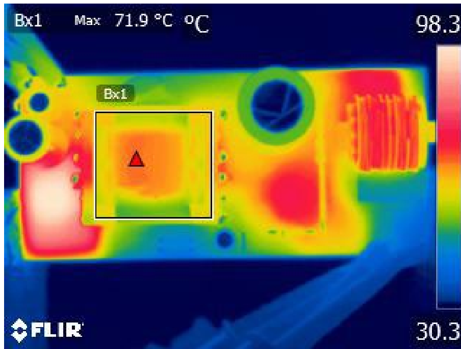
Figure 87 – 85 VAC 60 Hz. Top Side Discrete Component Thermals.
