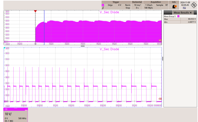
Figure 57 – 115 VAC 60 Hz. CH3: V_Sec Diode, 10 V / div., 10 ms / div. Zoom: 20 \mu s / div. Freewheel Diode Voltage (MAX) = 60.6 V
