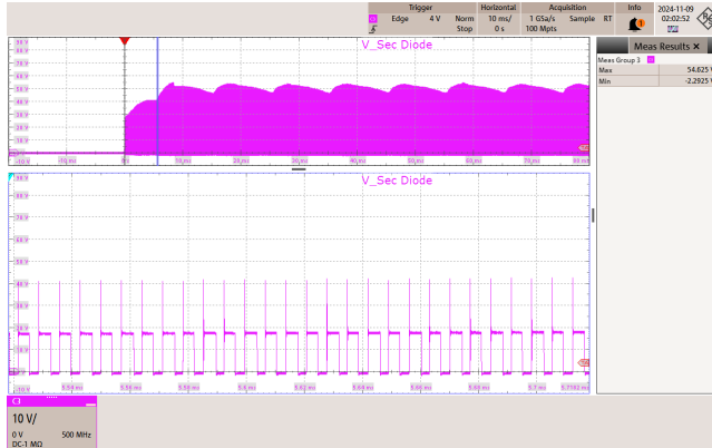
Figure 56 – 85 VAC 60 Hz. CH3: V_Sec Diode, 10 V / div., 10 ms / div. Zoom: 20 \mu s / div. Freewheel Diode Voltage (MAX) = 54.6 V
