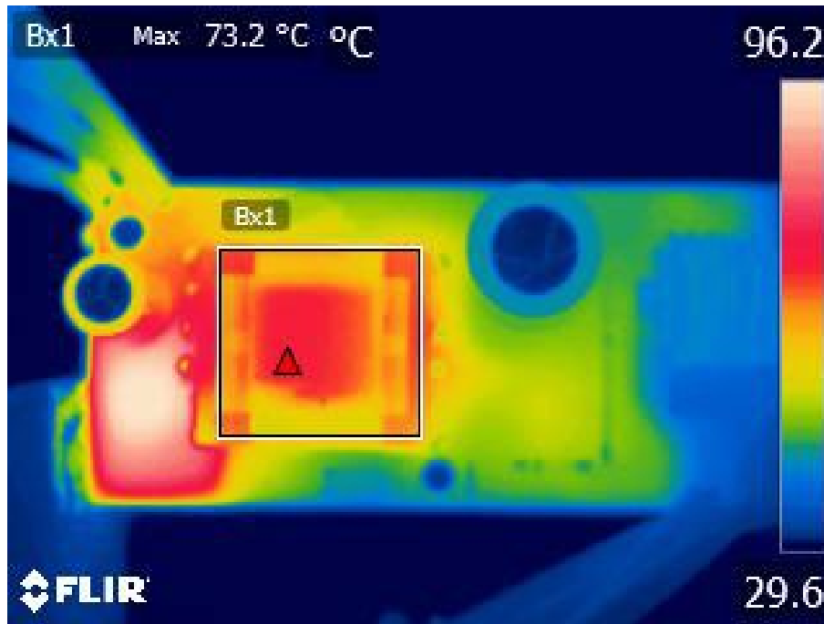
Figure 89 – 265 VAC 50 Hz. Top Side Discrete Component Thermals.
