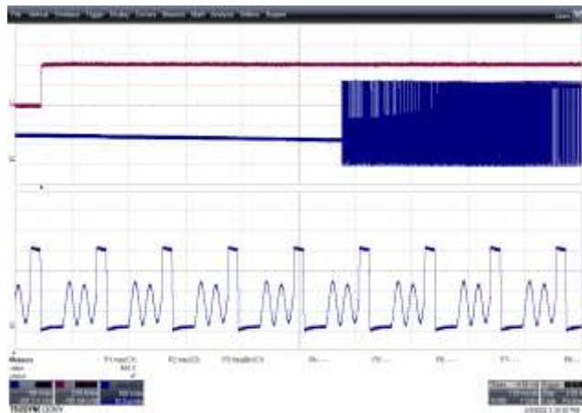
Figure 77 – PFC Boost Diode Reverse Voltage 198 VAC, 24 V 4.17 A Transient V_{DS} , 100 V / div., 5 us / div.(Zoom) V_{DMAX} : 404 V
