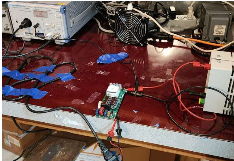
Figure 75 – Conducted EMI Test Set-up
