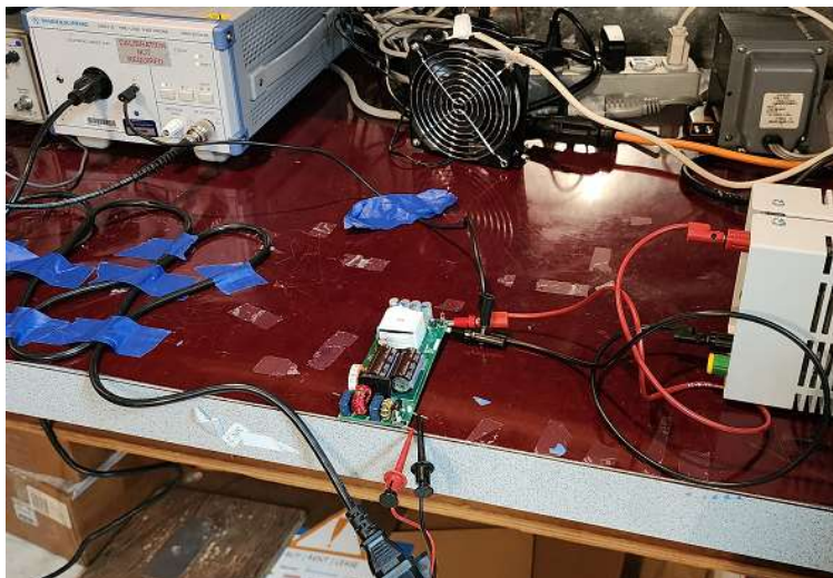
Figure 124 – Conducted EMI Test Set-up
