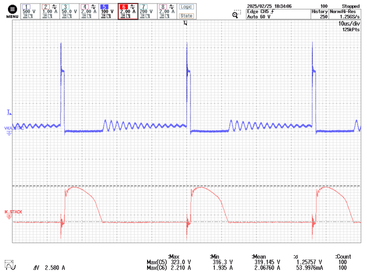
Figure 132 – 25.5 V Stack Diode Voltage and Current. 950 VDC, 25.5 V / Full Load, 24.7 V / Full Load, 85 °C Ambient. CH5: V_{KA}(25.5 \text{ V Diode}) , 100 V / div. CH6: I_{K}(25.5 \text{ V Diode}) , 2 A / div. Time: 10 \mu s / div.
