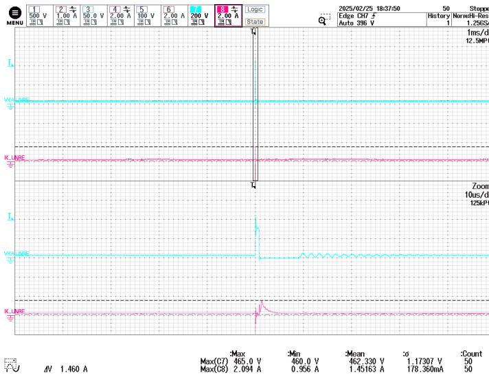
Figure 137 – 24.7 V Freewheeling Diode Voltage and Current. 950 VDC, 25.5 V / No Load, 24.7 V / No Load, 85 °C Ambient. CH7: V_{KA(24.7\text{ V Diode})} , 50 V / div. CH8: I_{K(24.7\text{ V Diode})} , 2 A / div. Time: 1 ms / div. (10 \mu s / div. Zoom)
