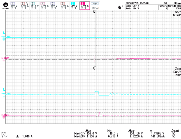
Figure 135 – 24.7 V Freewheeling Diode Voltage and Current. 250 VDC, 25.5 V / No Load, 24.7 V / No Load, 85 °C Ambient. CH7: V_{KA}(24.7 \text{ V Diode}) , 50 V / div. CH8: I_{K}(24.7 \text{ V Diode}) , 2 A / div. Time: 1 ms / div. (10 \mu s / div. Zoom)
