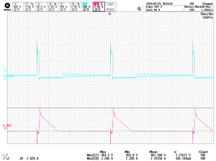
Figure 138 – 24.7 V Freewheeling Diode Voltage and Current. 950 VDC, 25.5 V / Full Load, 24.7 V / Full Load, 85 °C Ambient. CH7: V_{KA(24.7\text{ V Diode})} , 200 V / div. CH8: I_{K(24.7\text{ V Diode})} , 2 A / div. Time: 10 \mu s / div.
