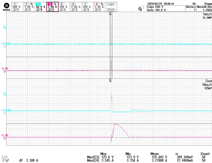
Figure 125 – SR FET Drain Voltage and Current. 950 VDC, 25.5 V / No Load, 24.7 V / No Load, 85 °C Ambient. CH3: V_{DS(SR FET)} , 50 V / div. CH4: I_{D(SR FET)} , 2 A / div. Time: 1 ms / div. (10 \mu s / div. Zoom)
