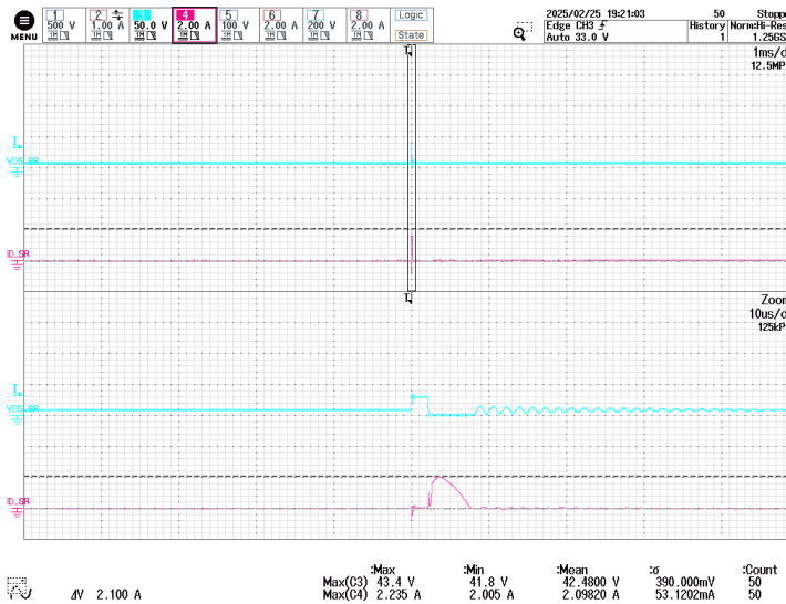
Figure 99 – SR FET Drain Voltage and Current. 250 VDC, 25.5 V / No Load, 24.7 V / No Load, 25 °C Ambient. CH3: V_{DS} (SR FET), 50 V / div. CH4: I_D (SR FET), 2 A / div. Time: 1 ms / div. (10 \mu s / div. Zoom)
