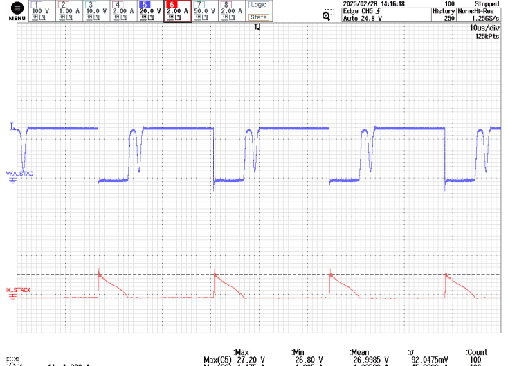
Figure 104 – 25.5 V Stack Diode Voltage and Current. 40 VDC, 25.5 V / Full Load, 24.7 V / Full Load, 25 °C Ambient. CH5: V_{KA} (25.5 V Diode), 100 V / div. CH6: I_k (25.5 v Diode), 2 A / div. Time: 10 \mu s / div.
