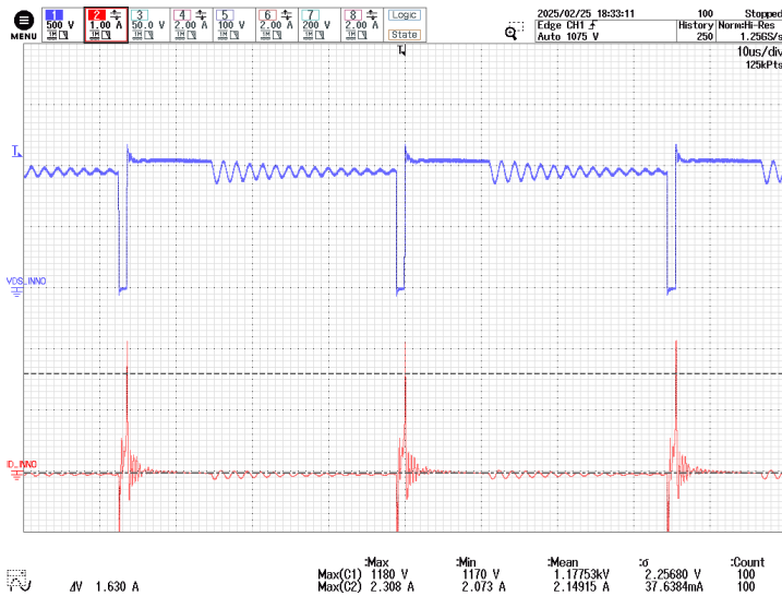
Figure 120 – INN3947FQ Drain Voltage and Current. 950 VDC, 25.5 V / Full Load, 24.7 V / Full Load, 85 °C Ambient. CH1: V_{DS(INNO)} , 500 V / div. CH2: I_{D(INNO)} , 1 A / div. Time: 10 \mu s / div.
