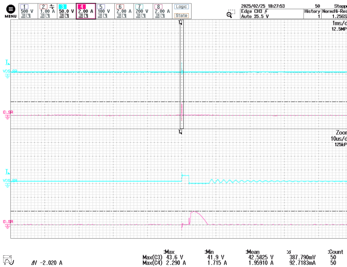
Figure 123 – SR FET Drain Voltage and Current. 250 VDC, 25.5 V / No Load, 24.7 V / No Load, 85 °C Ambient. CH3: V_{DS}(SR FET) , 50 V / div. CH4: I_D(SR FET) , 2 A / div. Time: 1 ms / div. (10 \mu s / div. Zoom)
