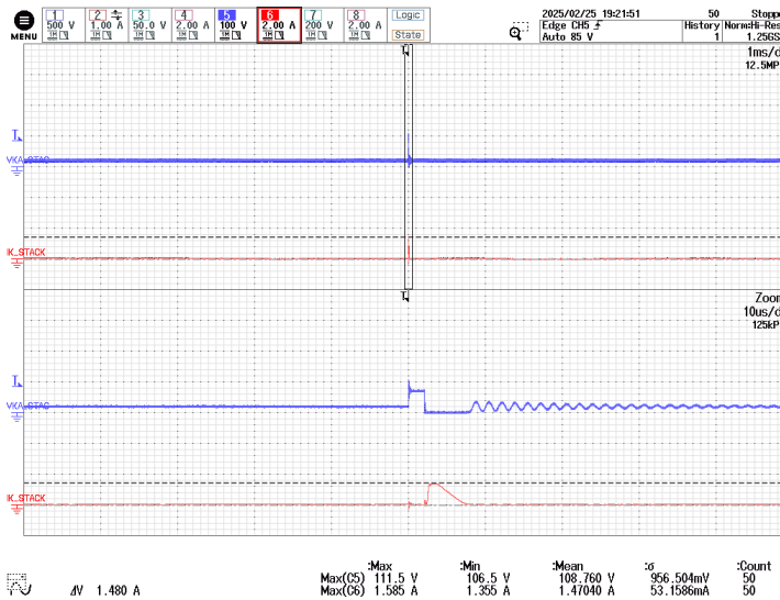
Figure 105 – 25.5 V Stack Diode Voltage and Current. 250 VDC, 25.5 V / No Load, 24.7 V / No Load, 25 °C Ambient. CH5: V_{KA} (25.5 V Diode), 20 V / div. CH6: I_k (25.5 V Diode), 2 A / div. Time: 1 ms / div. (10 \mu s / div. Zoom)
