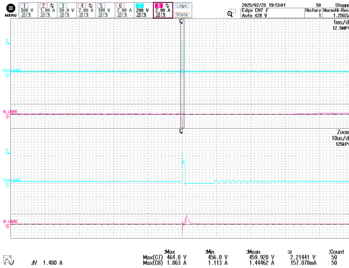
Figure 113 – 24.7 V Freewheeling Diode Voltage and Current. 950 VDC, 25.5 V / No Load, 24.7 V / No Load, 25 °C Ambient. CH7: V_{KA}(24.7 \text{ V Diode}) , 50 V / div. CH8: I_{K}(24.7 \text{ V Diode}) , 2 A / div. Time: 1 ms / div. (10 \mu s / div. Zoom)
