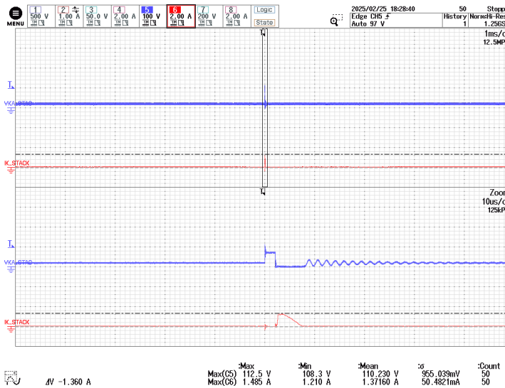
Figure 129 – 25.5 V Stack Diode Voltage and Current. 250 VDC, 25.5 V / No Load, 24.7 V / No Load, 85 °C Ambient. CH5: V_{KA}(25.5 \text{ V Diode}) , 20 V / div. CH6: I_{K}(25.5 \text{ V Diode}) , 2 A / div. Time: 1 ms / div. (10 \mu s / div. Zoom)
