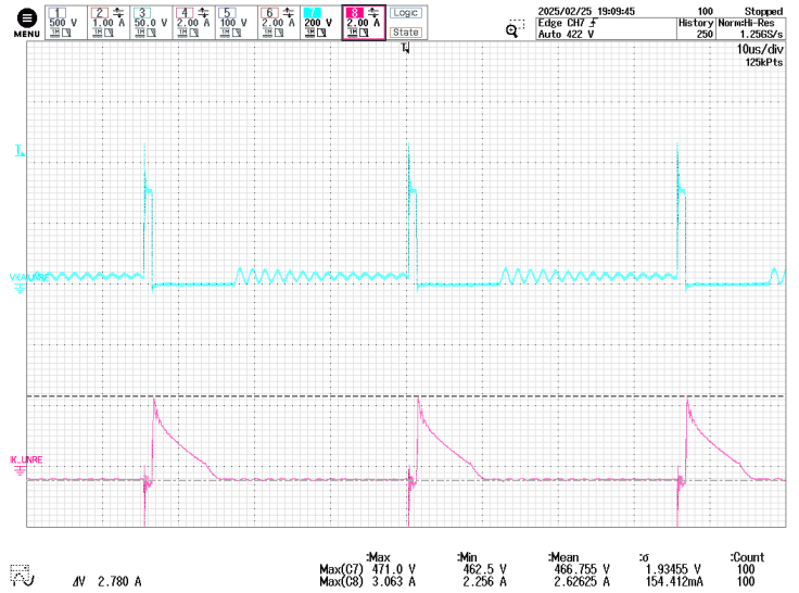
Figure 114 – 24.7 V Freewheeling Diode Voltage and Current. 950 VDC, 25.5 V / Full Load, 24.7 V / Full Load, 25 °C Ambient. CH7: V_{KA}(24.7 \text{ V Diode}) , 200 V / div. CH8: I_{K}(24.7 \text{ V Diode}) , 2 A / div. Time: 10 \mu s / div.
