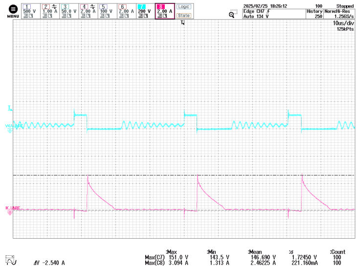
Figure 136 – 24.7 V Freewheeling Diode Voltage and Current. 250 VDC, 25.5 V / Full Load, 24.7 V / Full Load, 85 °C Ambient. CH7: V_{KA}(24.7 \text{ V Diode}) , 200 V / div. CH8: I_{K}(24.7 \text{ V Diode}) , 2 A / div. Time: 10 \mu s / div.
