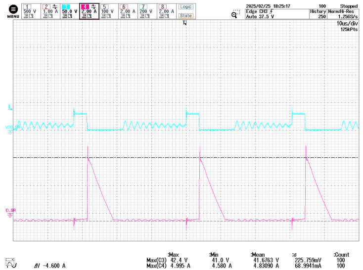
Figure 124 – SR FET Drain Voltage and Current. 250 VDC, 25.5 V / Full Load, 24.7 V / Full Load, 85 °C Ambient. CH3: V_{DS}(SR FET) , 50 V / div. CH4: I_D(SR FET) , 2 A / div. Time: 10 \mu s / div.
