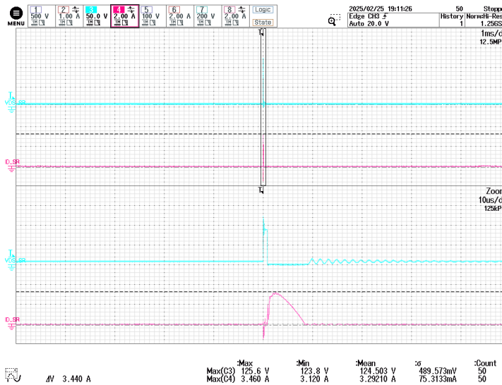
Figure 101 – SR FET Drain Voltage and Current. 950 VDC, 25.5 V / No Load, 24.7 V / No Load, 25 °C Ambient. CH3: V_{DS(SR FET)} , 50 V / div. CH4: I_D(SR FET) , 2 A / div. Time: 1 ms / div. (10 \mu s / div. Zoom)
