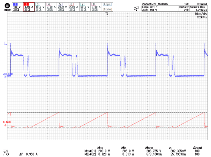
Figure 116 – INN3947FQ Drain Voltage and Current. 40 VDC, 25.5 V / Full Load, 24.7 V / Full Load, 85 °C Ambient. CH1: V_{DS(INNO)} , 500 V / div. CH2: I_{D(INNO)} , 1 A / div. Time: 10 \mu s / div.
