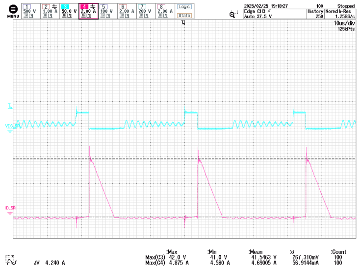
Figure 100 – SR FET Drain Voltage and Current. 250 VDC, 25.5 V / Full Load, 24.7 V / Full Load, 25 °C Ambient. CH3: V_{DS} (SR FET), 50 V / div. CH4: I_D (SR FET), 2 A / div. Time: 10 \mu s / div.
