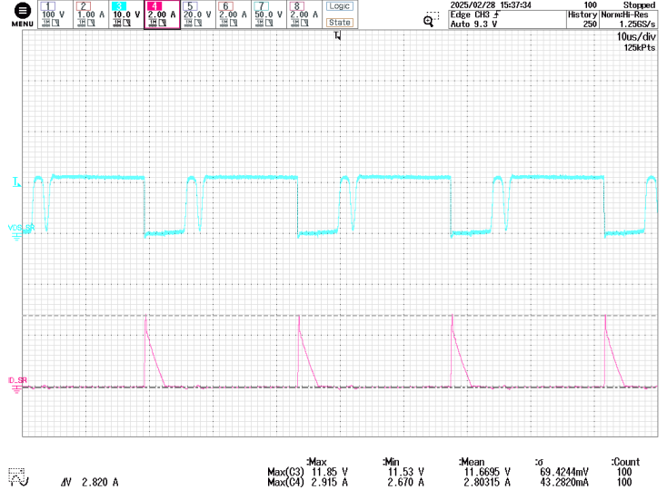
Figure 122 – SR FET Drain Voltage and Current. 40 VDC, 25.5 V / Full Load, 24.7 V / Full Load, 85 °C Ambient. CH3: V_{DS}(SR FET) , 50 V / div. CH4: I_D(SR FET) , 2 A / div. Time: 10 \mu s / div.
