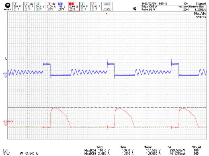
Figure 130 – 25.5 V Stack Diode Voltage and Current. 250 VDC, 25.5 V / Full Load, 24.7 V / Full Load, 85 °C Ambient. CH5: V_{KA}(25.5 \text{ V Diode}) , 100 V / div. CH6: I_{K}(25.5 \text{ V Diode}) , 2 A / div. Time: 10 \mu s / div.
