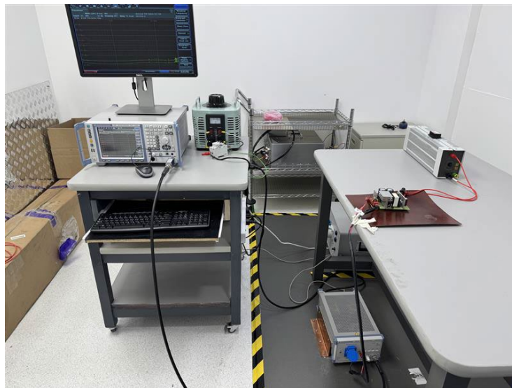
Figure 110 – EMI Test Set-up.
