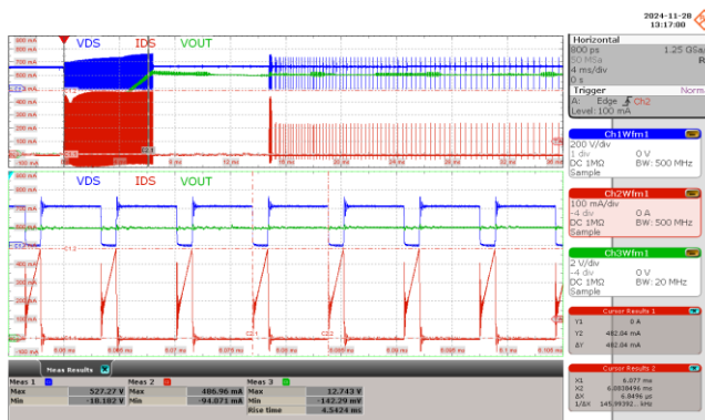
Figure 28 – 85 VAC 60 Hz. CH1: V_{DS} , 200 V / div., 4 ms / div. CH2: I_{DS} , 100 mA / div., 4 ms / div. CH3: V_{OUT} , 2 V / div., 4 ms / div Zoom: 5 \mu s / div. Drain Voltage (MAX) = 306 V Drain Current (MAX) = 475 mA
