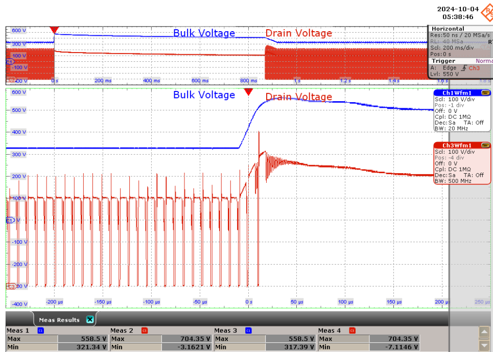
Figure 104 – 230 VAC, FL R_{Load} , -1 kV 180° surge event. CH 1: Bulk Voltage: 100 V / div., 200 ms / div. CH 2: Drain Voltage: 100 V / div., 200 ms / div. Zoom: 50 µs Drain Voltage, max = 704.4 V
