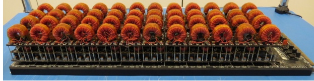
Figure 7 Custom test bed used to perform DHTOL on multiple 1250V InnoSwitch ICs in parallel at 125 °C.
