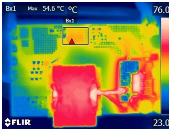
Figure 13 Steady-state thermals indicating temperature rise below 30 °C during continuous switching and a VDS(PK) of 1000 V.
