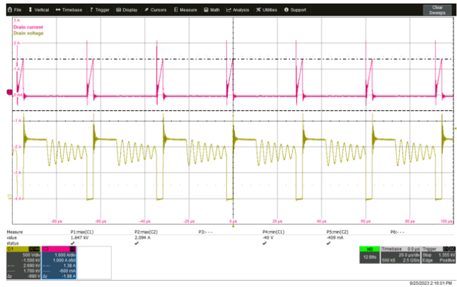
Figure 8 Drain voltage and current waveforms. Pink is the primary switch current (1 A per division); Brown is the VDS of the primary power switch (500 V per division); Time base is 20 us per division.
