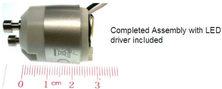
Figure 2 – Assembled Driver Inside GU10 Base.
