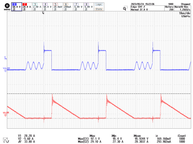
Figure 64 – SR FET Drain Voltage and Current. 900 V DC , 6.37 A Load, 25 °C Ambient. CH1: V DS,SRFET , 50 V / div. CH2: I D,SRFET , 20 A / div. Time: 10 μs / div.
