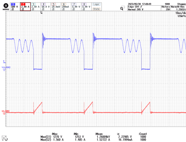
Figure 59 – InnoSwitch3-AQ Drain Voltage and Current. 800 V DC , 6.37 A Load, 25 °C Ambient. CH1: V DS,INNO , 500 V / div. CH2: I D,INNO , 2 A / div. Time: 10 μs / div.
