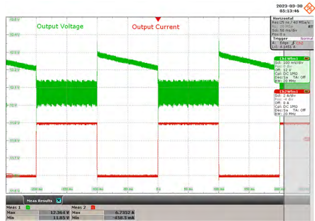
Figure 29 – 115 VAC 60 Hz. I_o = 0\text{ A} - 6\text{ A} (0 - 100%) Load Step. CH1: Output Voltage: 100 mV / div., 50 ms / div. CH2: Output Current: 2 A / div., 50 ms / div. V_{O1\_MAX} : 12.4 V. V_{O1\_MIN} : 11.9 V.
