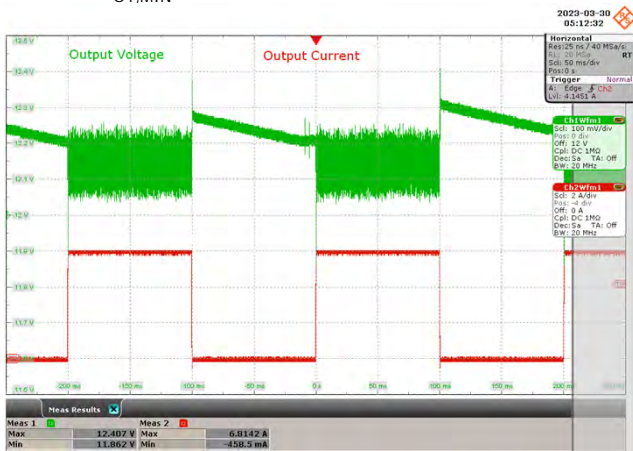
Figure 30 – 230 VAC 50 Hz. I_o = 0\text{ A} - 6\text{ A} (0 - 100%) Load Step. CH1: Output Voltage: 100 mV / div., 50 ms / div. CH2: Output Current: 2 A / div., 50 ms / div. V_{O1\_MAX} : 12.4 V. V_{O1\_MIN} : 11.9 V.
