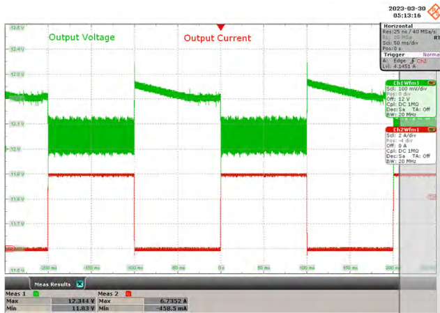
Figure 28 – 90 VAC 60 Hz. I_o = 0\text{ A} - 6\text{ A} (0 - 100%) Load Step. CH1: Output Voltage: 100 mV / div., 50 ms / div. CH2: Output Current: 2 A / div., 50 ms / div. V_{O1\_MAX} : 12.3 V. V_{O1\_MIN} : 11.8 V.
