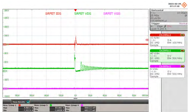
Figure 51 – 265 VAC, I_o = 0 A (No-Load).
