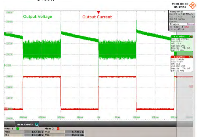
Figure 31 – 265 VAC 50 Hz. I_o = 0\text{ A} - 6\text{ A} (0 - 100%) Load Step. CH1: Output Voltage: 100 mV / div., 50 ms / div. CH2: Output Current: 2 A / div., 50 ms / div. V_{O1\_MAX} : 12.4 V. V_{O1\_MIN} : 11.9 V.
