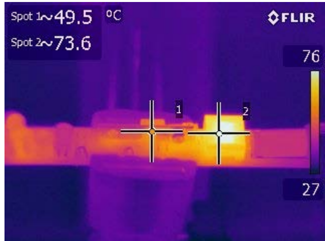
Figure 20 – 115 VAC, Full Load. Spot 1: LYT4214E. Spot 2: Transformer.
