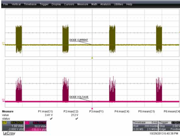
Figure 53 – 195 VAC, 50 Hz. Upper: I_{D7} , 1 A / div. Lower: V_{D7} , 50 V, 200 ms / div.
