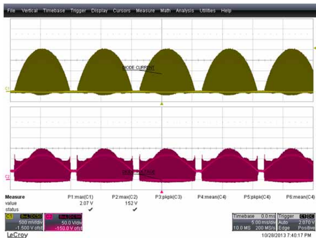
Figure 47 – 195 VAC, 50 Hz. Upper: I_{D7} , 0.5 A / div. Lower: V_{D7} , 50 V, 5 ms / div.
