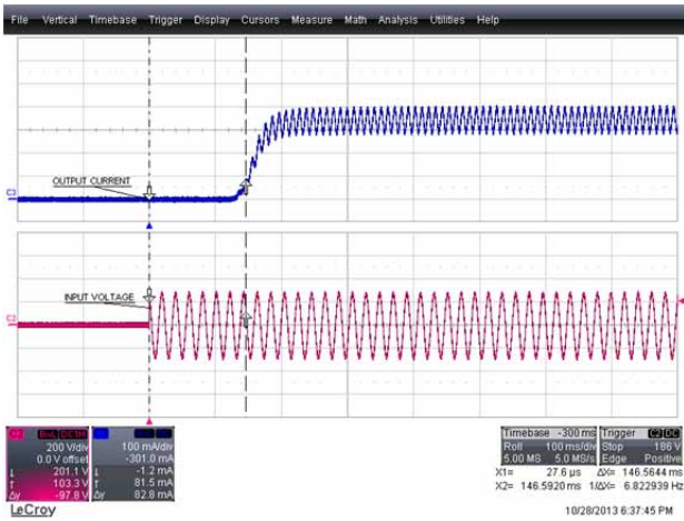
Figure 31 – 195 VAC, 50 Hz. Upper: I_{OUT} , 100 mA / div. Lower: V_{IN} , 200 V, 100 ms / div. Start-up Time: 146 ms
