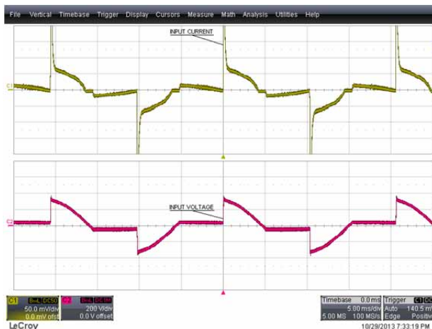
Figure 60 – 90° Conduction Angle. Upper: I_{IN} , 50 mA / div. Lower: V_{IN} , 200 V, 5 ms / div.
