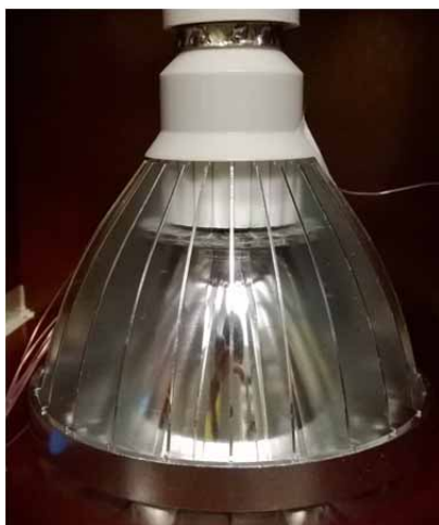
Figure 23 – Actual LED Enclosure Used in Thermal Verification.
