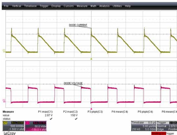
Figure 48 – 195 VAC, 50 Hz. Upper: I_{D7} , 0.5 A / div. Lower: V_{D7} , 50 V / div., 5 \mu s / div.
