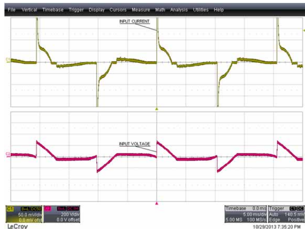
Figure 61 – 60° Conduction Angle. Upper: I_{IN} , 50 mA / div. Lower: V_{IN} , 200 V, 5 ms / div.
