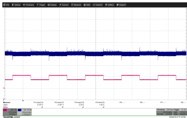
Figure 49 – Transient Response. 85 VAC, 3.3 V, 1.5 – 2.25 A Load Step. V_{MIN} : 3.181 V, V_{MAX} : 3.415 V. Upper: V_{OUT} , 0.2 V / div., 50 ms / div. Lower: I_{LOAD} , 2 A / div.
