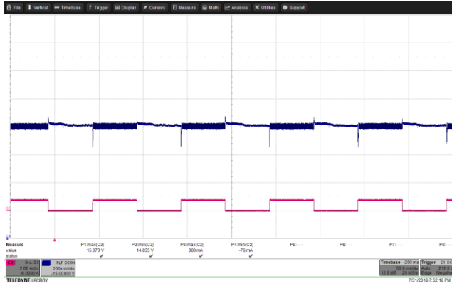
Figure 69 – Transient Response. 85 VAC, 15.0 V, 0 – 0.75 A Load Step. V_{MIN} : 14.867 V, V_{MAX} : 15.060 V. Upper: V_{OUT} , 0.2 V / div., 50 ms / div. Lower: I_{LOAD} , 2 A / div.
