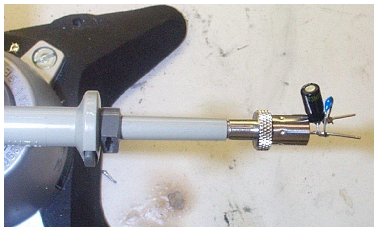
Figure 105 – Oscilloscope Probe with Probe Master ( www.probemaster.com ) 4987A BNC Adapter. (Modified with wires for ripple measurement, and two parallel decoupling capacitors added)
