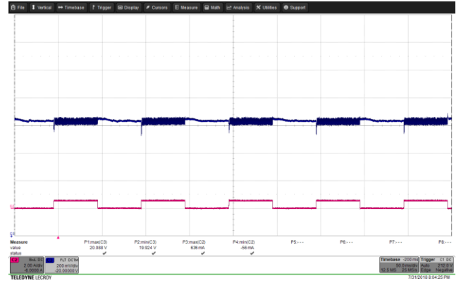
Figure 78 – Transient Response. 265 VAC, 20.0 V, 0 – 0.56 A Load Step. V_{MIN} : 19.924 V, V_{MAX} : 20.088 V. Upper: V_{OUT} , 0.2 V / div., 50 ms / div. Lower: I_{LOAD} , 2 A / div.
