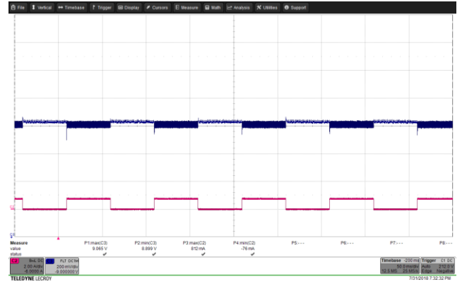
Figure 62 – Transient Response. 265 VAC, 9.0 V, 0 – 0.75 A Load Step. V_{MIN} : 8.899 V, V_{MAX} : 9.065 V. Upper: V_{OUT} , 0.2 V / div., 50 ms / div. Lower: I_{LOAD} , 2 A / div.
