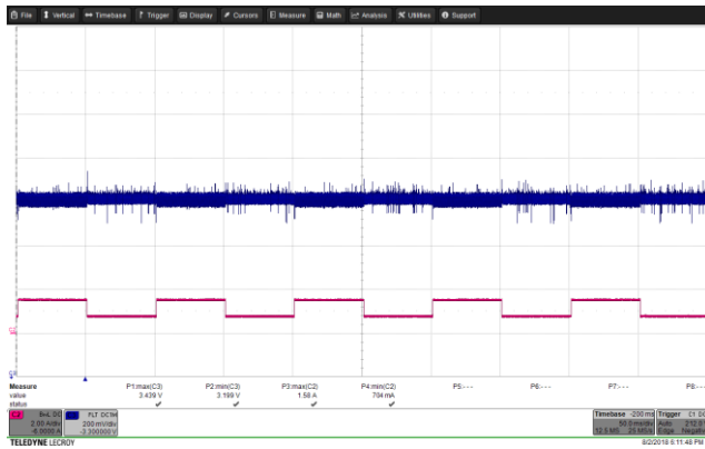
Figure 47 – Transient Response. 85 VAC, 3.3 V, 0.75 – 1.5 A Load Step. V_{MIN} : 3.199 V, V_{MAX} : 3.439 V. Upper: V_{OUT} , 0.2 V / div., 50 ms / div. Lower: I_{LOAD} , 2 A / div.
