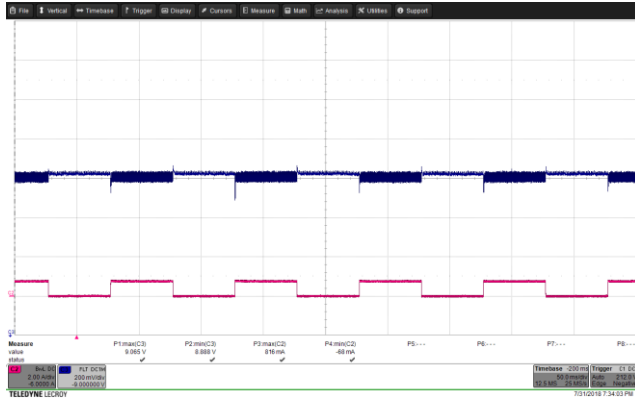
Figure 61 – Transient Response. 85 VAC, 9.0 V, 0 – 0.75 A Load Step. V_{MIN} : 8.888 V, V_{MAX} : 9.065 V. Upper: V_{OUT} , 0.2 V / div., 50 ms / div. Lower: I_{LOAD} , 2 A / div.
