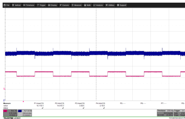
Figure 76 – Transient Response. 265 VAC, 15 V, 2.25 – 3 A Load Step. V_{MIN} : 14.915 V, V_{MAX} : 15.118 V. Upper: V_{OUT} , .2 V / div., 50 ms / div. Lower: I_{LOAD} , 2 A / div.
