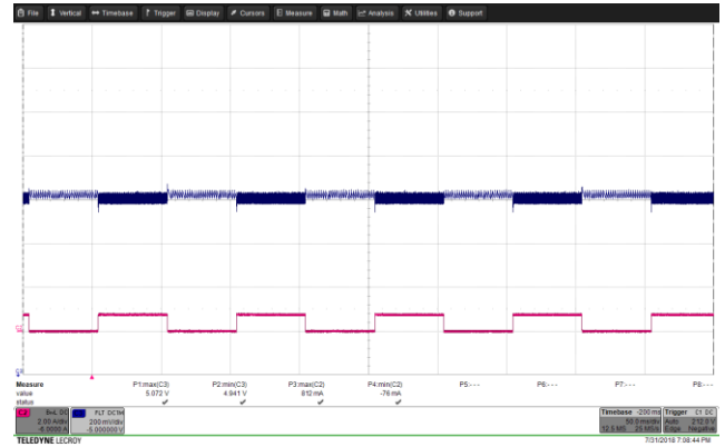
Figure 54 – Transient Response. 265 VAC, 5.0 V, 0 – 0.75 A Load Step. V_{MIN} : 4.941 V, V_{MAX} : 5.072 V. Upper: V_{OUT} , 0.2 V / div., 50 ms / div. Lower: I_{LOAD} , 2 A / div.
