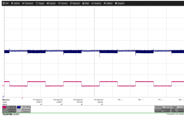
Figure 53 – Transient Response. 85 VAC, 5.0 V, 0 – 0.75 A Load Step. V_{MIN} : 4.899 V, V_{MAX} : 5.060 V. Upper: V_{OUT} , 0.2 V / div., 50 ms / div. Lower: I_{LOAD} , 2 A / div.
