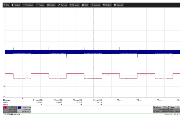
Figure 66 – Transient Response. 265 VAC, 9.0 V, 1.5 – 2.25 A Load Step. V_{MIN} : 8.913 V, V_{MAX} : 9.103 V. Upper: V_{OUT} , 0.2 V / div., 50 ms / div. Lower: I_{LOAD} , 2 A / div.
