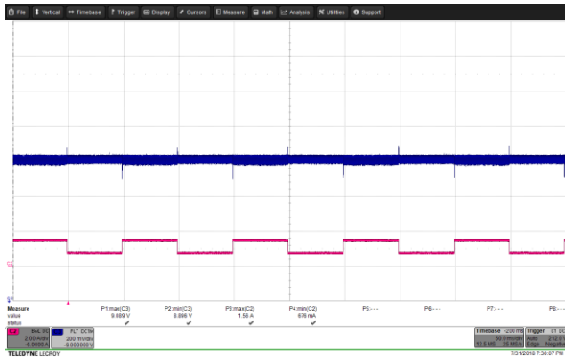
Figure 63 – Transient Response. 85 VAC, 9.0 V, 0.75 – 1.5 A Load Step. V_{MIN} : 8.896 V, V_{MAX} : 9.089 V. Upper: V_{OUT} , 0.2 V / div., 50 ms / div. Lower: I_{LOAD} , 2 A / div.
