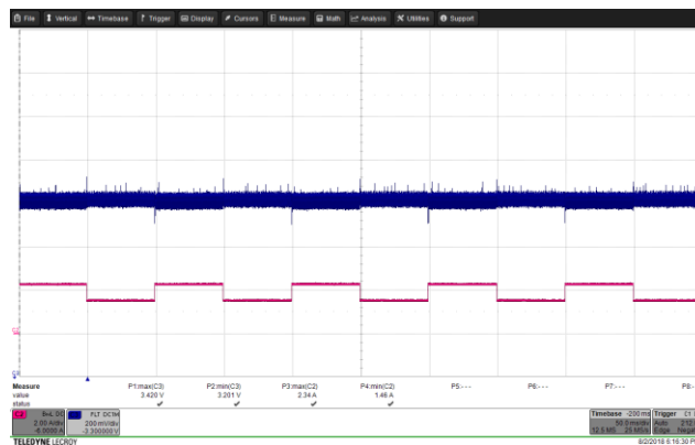
Figure 50 – Transient Response. 265 VAC, 3.3 V, 1.5 – 2.25 A Load Step. V_{MIN} : 3.201 V, V_{MAX} : 3.420 V. Upper: V_{OUT} , 0.2 V / div., 50 ms / div. Lower: I_{LOAD} , 2 A / div.
