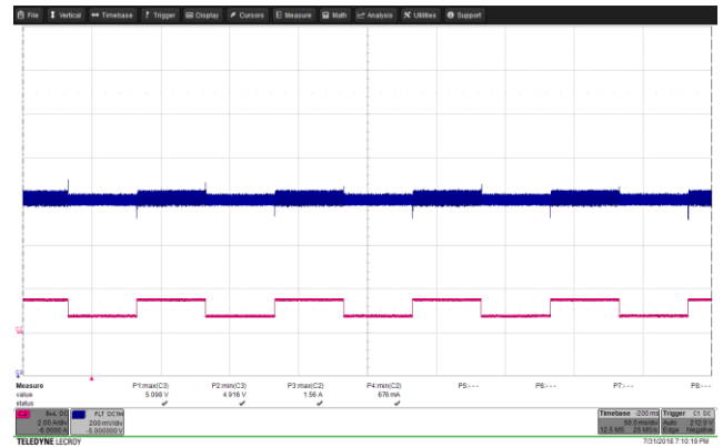
Figure 56 – Transient Response. 265 VAC, 5.0 V, 0.75 – 1.5 A Load Step. V_{MIN} : 4.961 V, V_{MAX} : 5.098 V. Upper: V_{OUT} , 0.2 V / div., 50 ms / div. Lower: I_{LOAD} , 2 A / div.
