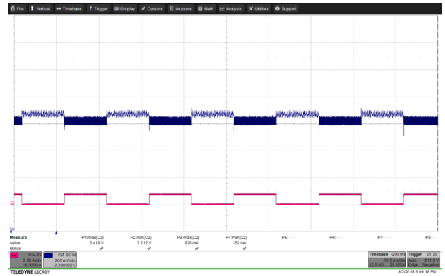
Figure 46 – Transient Response. 265 VAC, 3.3 V, 0 – 0.75 A Load Step. V_{MIN} : 3.212 V, V_{MAX} : 3.419 V. Upper: V_{OUT} , 0.2 V / div., 50 ms / div. Lower: I_{LOAD} , 2 A / div.
