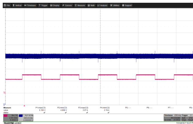
Figure 60 – Transient Response. 265 VAC, 5.0 V, 2.25 – 3 A Load Step. V_{MIN} : 4.908 V, V_{MAX} : 5.100 V. Upper: V_{OUT} , .2 V / div., 50 ms / div. Lower: I_{LOAD} , 2 A / div.
