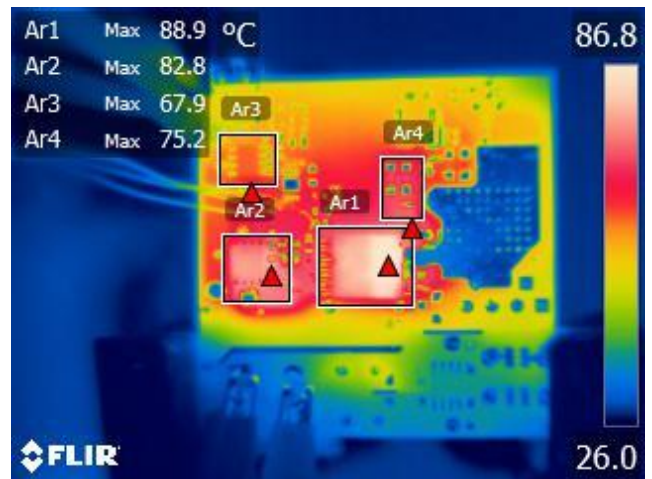
Figure 46 – Bottom Side Thermal Image.
