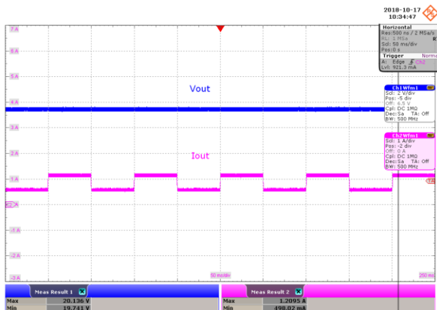
Figure 119 – Dynamic Load Response. 85 VAC, 20 V, 0.56 – 1.125 A Load Step. V_{MAX} : 20.13 V, V_{MIN} : 19.74 V. Upper: V_{OUT} , 2 V / div., 50 ms / div. Lower: I_{LOAD} , 1 A / div.
