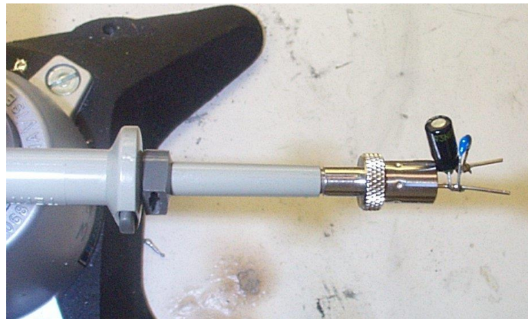
Figure 63 – Oscilloscope Probe with Probe Master ( www.probemaster.com ) 4987A BNC Adapter. (Modified with wires for ripple measurement, and two parallel decoupling capacitors added)
