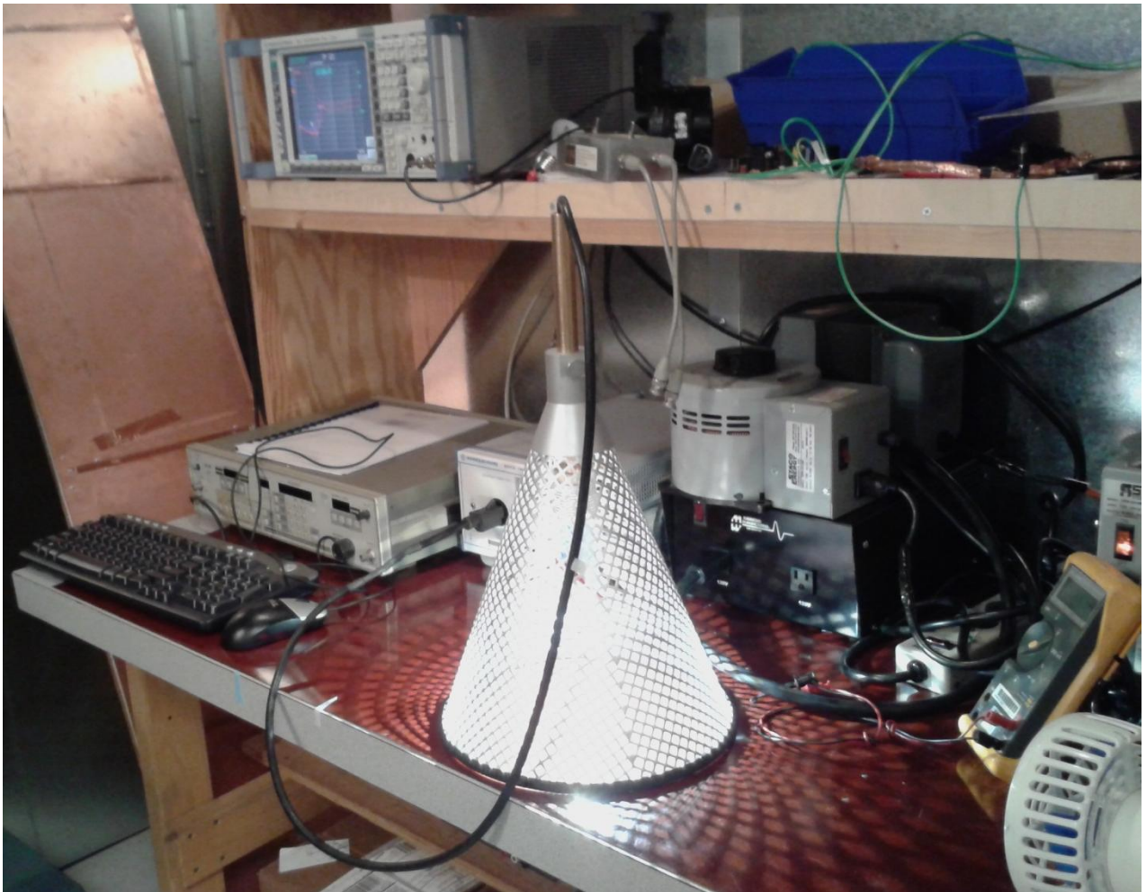
Figure 42 – The Retrofit Lamp was Verified Inside a Conical Metal Cone as per EN55015.
