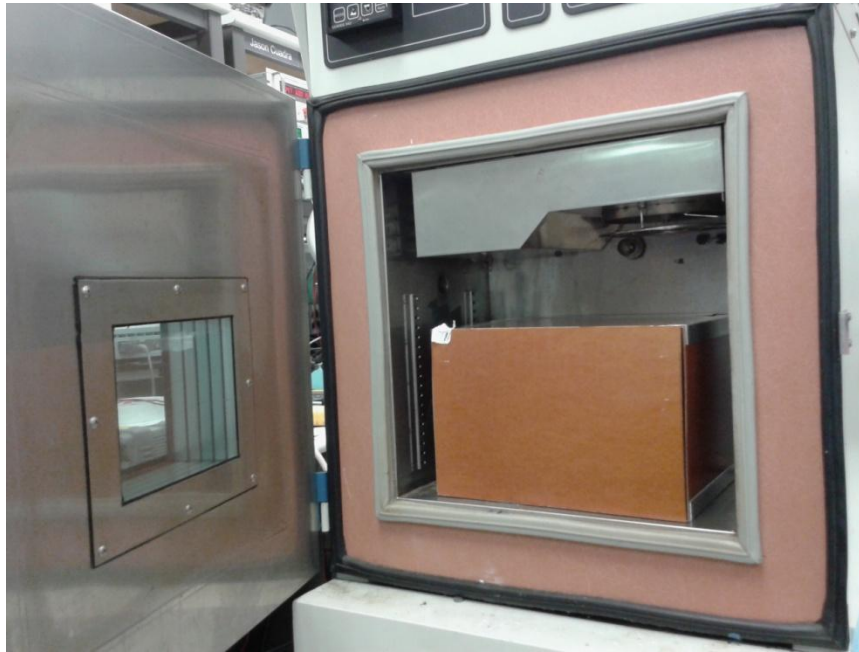
Figure 9 – Thermal Chamber Set-up Showing Box Used to Prevent Airflow Over UUT. Open Frame Set-up Measurement.
