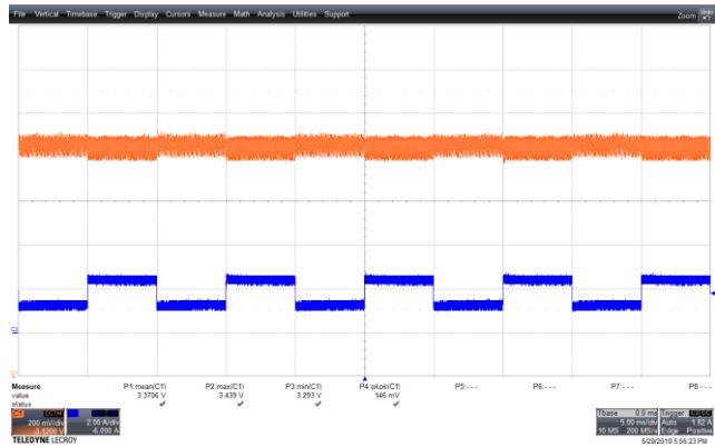
Figure 66 – Transient Response. 265 VAC, 3.3 V, 1.25 – 2.5 A Load Step. V_{MIN} : 3.293 V, V_{MAX} : 3.439 V. Upper: V_{OUT} , 0.2 V / div., 5 ms / div. Lower: I_{LOAD} , 2 A / div.
