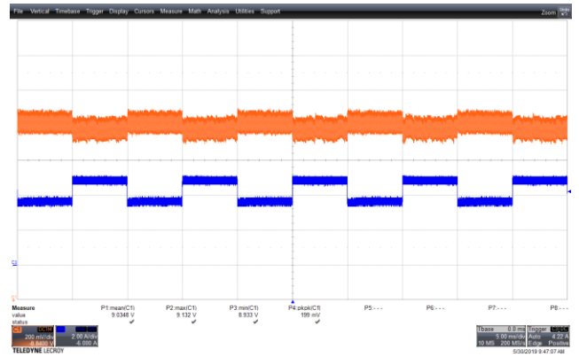
Figure 86 – Transient Response. 265 VAC, 9 V, 3.75 – 5 A Load Step. V_{MIN} : 8.933 V, V_{MAX} : 9.132 V. Upper: V_{OUT} , 0.2 V / div., 5 ms / div. Lower: I_{LOAD} , 2 A / div.
