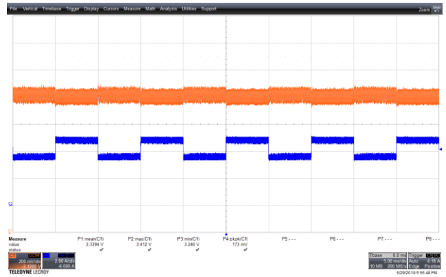
Figure 70 – Transient Response. 265 VAC, 3.3 V, 3.75 – 5 A Load Step. V_{MIN} : 3.240 V, V_{MAX} : 3.412 V. Upper: V_{OUT} , 0.2 V / div., 5 ms / div. Lower: I_{LOAD} , 2 A / div.
