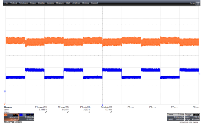
Figure 68 – Transient Response. 265 VAC, 3.3 V, 2.5 – 3.75 A Load Step. V_{MIN} : 3.253 V, V_{MAX} : 3.426 V. Upper: V_{OUT} , 0.2 V / div., 5 ms / div. Lower: I_{LOAD} , 2 A / div.
