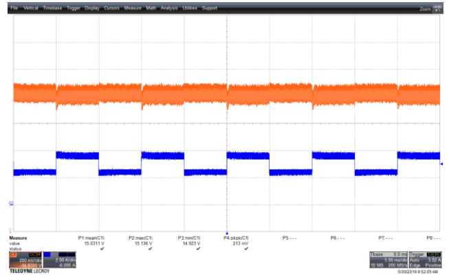
Figure 92 – Transient Response. 265 VAC, 15 V, 2.5 – 3.75 A Load Step. V_{MIN} : 14.923 V, V_{MAX} : 15.136 V. Upper: V_{OUT} , 0.2 V / div., 5 ms / div. Lower: I_{LOAD} , 2 A / div.
