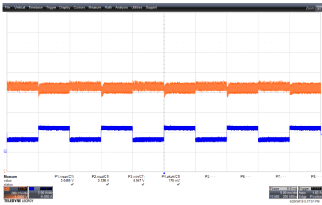
Figure 73 – Transient Response. 90 VAC, 5 V, 1.25 – 2.5 A Load Step. V_{MIN} : 4.947 V, V_{MAX} : 5.126 V. Upper: V_{OUT} , 0.2 V / div., 5 ms / div. Lower: I_{LOAD} , 2 A / div.
