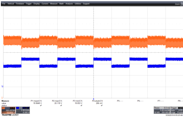
Figure 101 – Transient Response. 90 VAC, 20 V, 3.75 – 5 A Load Step. V_{MIN} : 19.853 V, V_{MAX} : 20.119 V. Upper: V_{OUT} , 0.2 V / div., 5 ms / div. Lower: I_{LOAD} , 2 A / div.
