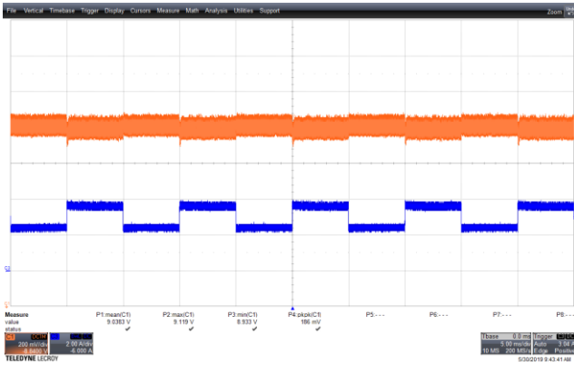
Figure 83 – Transient Response. 90 VAC, 9 V, 2.5 – 3.75 A Load Step. V_{MIN} : 8.933 V, V_{MAX} : 9.119 V. Upper: V_{OUT} , 0.2 V / div., 5 ms / div. Lower: I_{LOAD} , 2 A / div.
