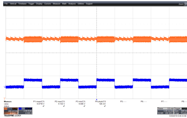
Figure 80 – Transient Response. 265 VAC, 9 V, 0 – 1.25 A Load Step. V_{MIN} : 9.006 V, V_{MAX} : 9.132 V. Upper: V_{OUT} , 0.2 V / div., 5 ms / div. Lower: I_{LOAD} , 2 A / div.
