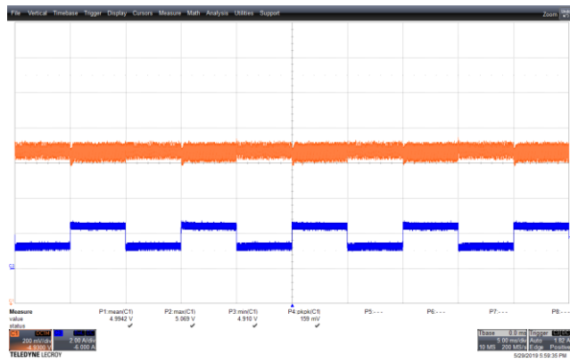
Figure 74 – Transient Response. 265 VAC, 5 V, 1.25 – 2.5 A Load Step. V_{MIN} : 4.91 V, V_{MAX} : 5.069 V. Upper: V_{OUT} , 0.2 V / div., 5 ms / div. Lower: I_{LOAD} , 2 A / div.
