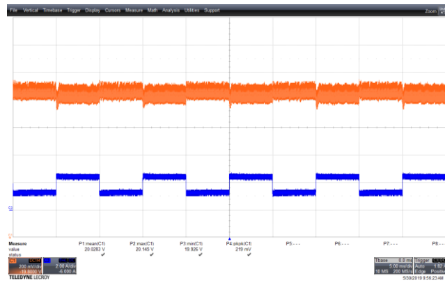
Figure 98 – Transient Response. 265 VAC, 20 V, 1.25 – 2.5 A Load Step. V_{MIN} : 19.926 V, V_{MAX} : 20.145 V. Upper: V_{OUT} , 0.2 V / div., 5 ms / div. Lower: I_{LOAD} , 2 A / div.
