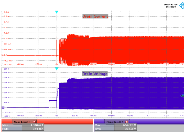
Figure 63 – 100 VAC, 36 V LED Load Panel. Upper: I_{DRAIN} , 400 mA / div. Lower: V_{DRAIN} , 100 V / div., 200 ms / div.
