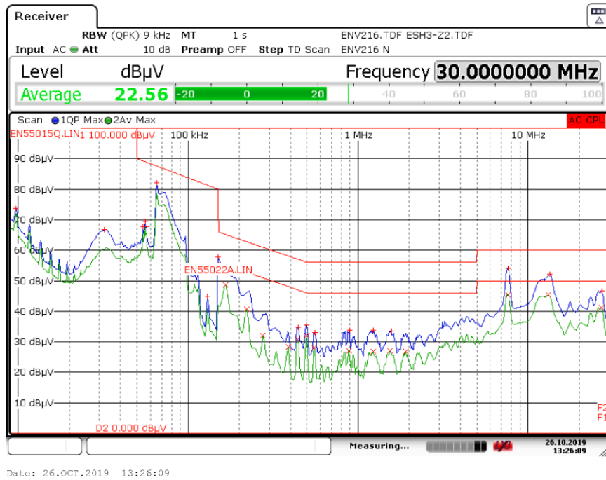
Figure 78 – Conducted EMI QP Scan at 36 V LED Load Panel, 230 VAC, 60 Hz, and EN55015 B Limits.
