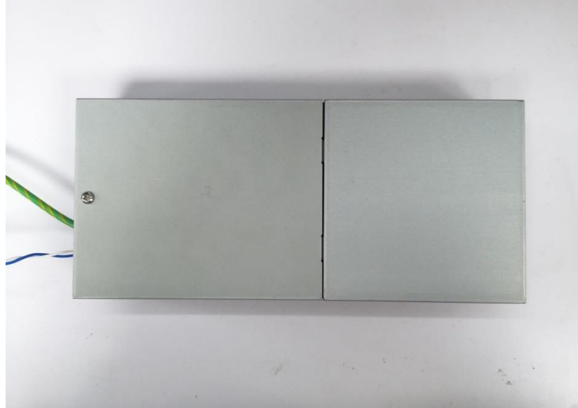
Figure 31 – Test Set-up Picture Thermal Inside Enclosure 50 °C - Closed Frame.
