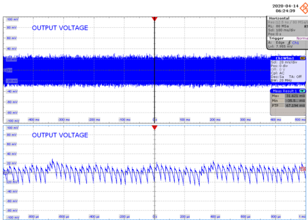
Figure 71 – 400 VDC Input. CH1: V_{OUT} , 20 mV / div., 100 ms / div. Zoom: 200 \mu s / div. 15 V Output Ripple = 67.194 mV.
