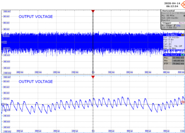
Figure 89 – 60 VDC Input. CH1: V_{OUT} , 20 mV / div., 100 ms / div. Zoom: 200 \mu s / div. 15 V Output Ripple = 79.842 mV.
