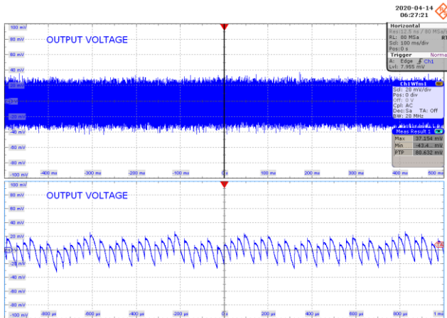
Figure 79 – 400 VDC Input. CH1: V_{OUT} , 20 mV / div., 100 ms / div. Zoom: 200 \mu s / div. 15 V Output Ripple = 80.632 mV.
