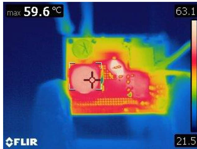
Figure 119 – Thermal Performance at 550 VDC Input. L1 = 59.6 °C
