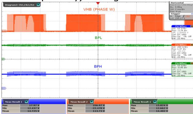
Figure 31 – INL and /INH Signal at Light Load. CH2: V_{HB\_PHASEW} , 200 V / div. CH4: V_{BPL} , 10 V / div. CH1: V_{BPH} , 10 V / div. Time Scale: 2 ms / div. BPL Average Voltage = 14.40 V. BPH Average Voltage = 14.72 V.
