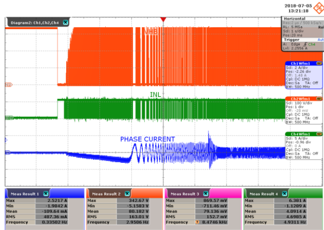
Figure 17 – Motor Start-up at 100 W Load. CH2: V_{HB} , 100 V / div. CH4: V_{INL} , 5 V / div. CH1: I_{PHASE\_CURRENT} , 2 A / div. Time Scale: 1 s / div. Maximum Phase Peak Current = 2.52 A PK . Maximum VHB Peak Voltage = 342.67 V PK .
