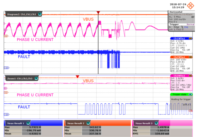
Figure 65 – HS OCP, R_{XL}/R_{XH} = 115\text{ k}\Omega , I_{LIM} = 1.1\text{ A} . CH2: V_{BUS} , 100 V / div. CH2: I_{PHASE} , 1 A / div. CH1: V_{FAULT} , 2 V / div. Time Scale: 100 ms / div. Time Scale (Zoomed Area): 100 \mu s / div. FAULT Flag Reading = 0000001.
