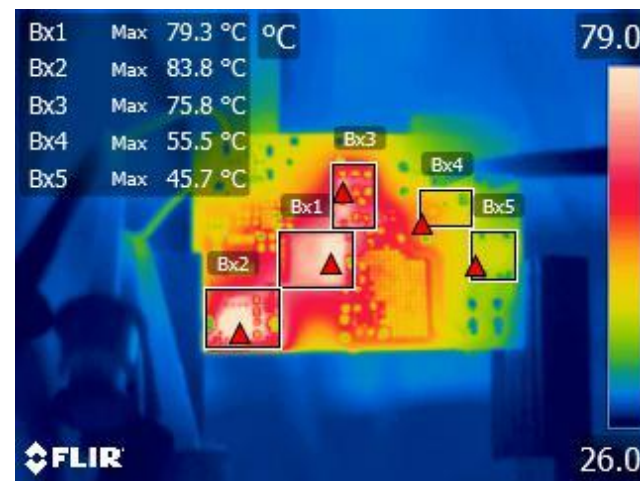
Figure 36 – Bottom Side Thermal Image. Bx1: InnoSwitch3-Pro = 79.3 °C. Bx2: SR FET = 83.8 °C. Bx3: Primary Snubber = 75.8 °C. Bx4: Thermistor RT1, PCB = 55.5 °C. Bx5: Bridge Rectifier = 45.7 °C.
