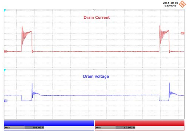
Figure 75 – 90 VAC, 60 V LED Load, Start-up. Upper: I_{DRAIN} , 500 mA / div. Lower: V_{DRAIN} , 100 V / div., 2 \mu s / div. Peak I_{DRAIN} : 2.22 A. Peak V_{DRAIN} : 381.06 V.
