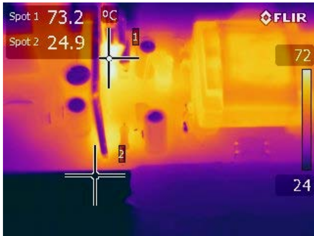
Figure 25 – 132 V VAC, Full load Spot 1: LYT4315E (U1): 73.2 °C.
