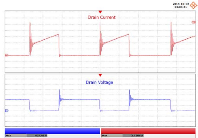
Figure 67 – 90 VAC, 60 V LED Load. Upper: I_{DRAIN} , 500 mA / div. Lower: V_{DRAIN} , 100 V / div., 2 \mu s / div. Peak I_{DRAIN} : 2.71 A. Peak V_{DRAIN} : 407.5 V.
