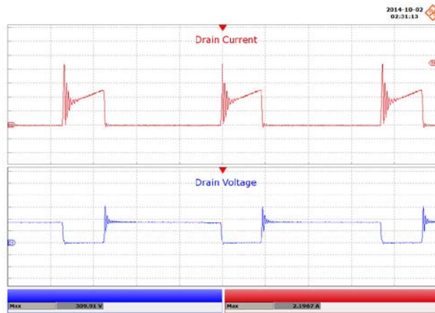
Figure 71 – 90 VAC, 30 V LED Load. Upper: I_{DRAIN} , 500 mA / div. Lower: V_{DRAIN} , 100 V / div., 2 \mu s / div. Peak I_{DRAIN} : 2.2 A. Peak V_{DRAIN} : 309.9 V.
