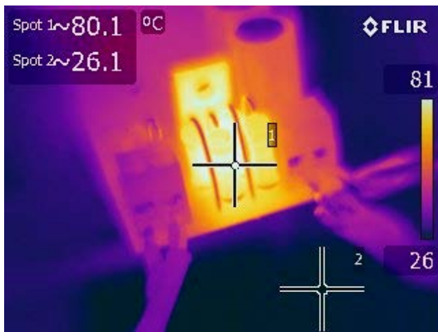
Figure 40 – 90 V VAC, 30 V LED Load, 0 V Dim. Spot 1: Pre-Load Resistors (R51-R60): 80.1 °C.
