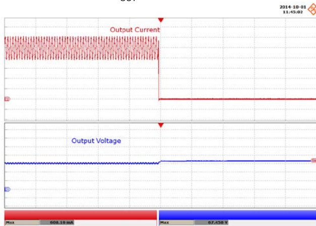
Figure 92 – 90 VAC, 60 V LED Load, Running Open Load. Upper: I_{OUT} , 100 mA / div. Lower: V_{OUT} , 20 V / div., 100 ms / div. Peak I_{OUT} : 608.16 mA. Peak V_{OUT} : 67.46 V.
