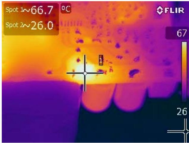
Figure 32 – 115 V VAC, Full Load. Spot 1: Output Diode (D16): 66.7 °C.
