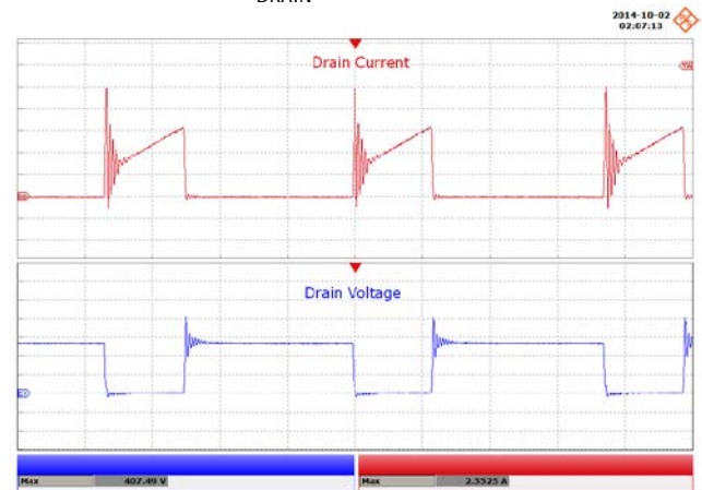
Figure 67 – 90 VAC, 60 V LED Load. Upper: I_{DRAIN} , 500 mA / div. Lower: V_{DRAIN} , 100 V / div., 2 \mu s / div. Peak I_{DRAIN} : 2.71 A. Peak V_{DRAIN} : 407.5 V.
