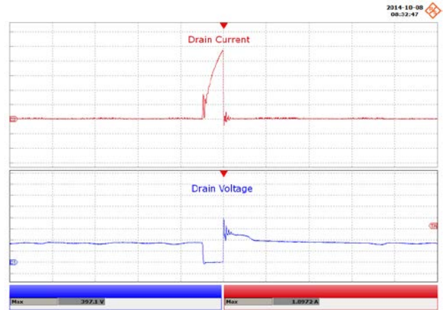
Figure 77 – 132 VAC, 60 V LED Load, Start-up. Upper: I_{DRAIN} , 500 mA / div. Lower: V_{DRAIN} , 100 V / div., 2 \mu s / div. Peak I_{DRAIN} : 1.89 A. Peak V_{DRAIN} : 397.1 V.
