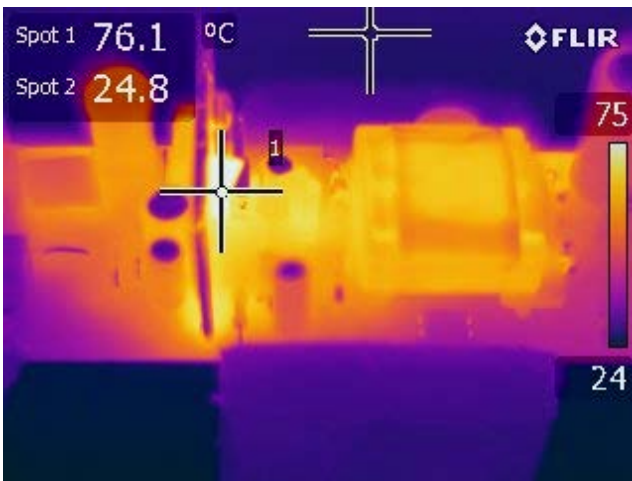
Figure 30 – 115 V VAC, Full Load. Spot 1: LYT4315E (U1): 76.1 °C.
