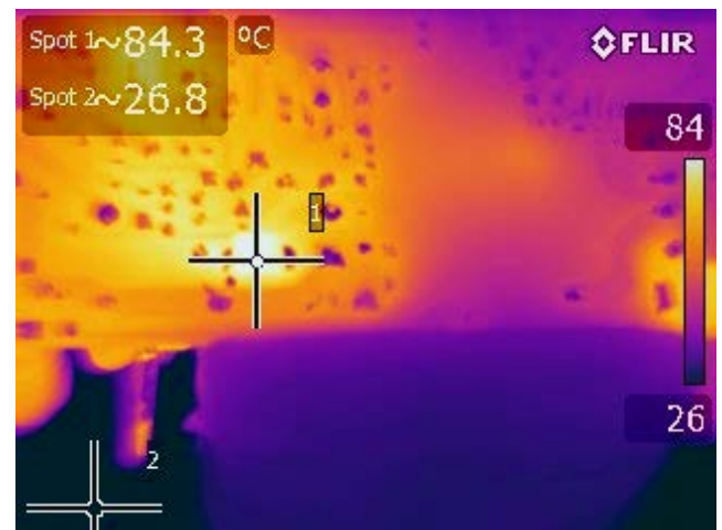
Figure 38 – 90 V VAC, Full Load. Spot 1: Blocking Diode (D7): 84.3 °C.
