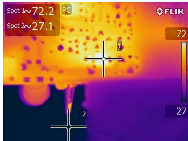
Figure 28 – 132 V VAC, Full Load. Spot 1: Blocking Diode (D7): 72.2 °C.
